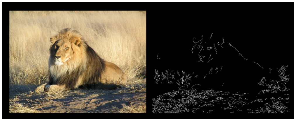
Figure 1.1 Visualize Feature Map after Convolution Operation. The original lion image is shown on the left. The feature map after convolution operation with edge detection kernel is shown on the right.
