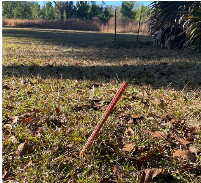
Figure 38. Rebar marking a GCP location that has been damaged and is missing its safety cap.
