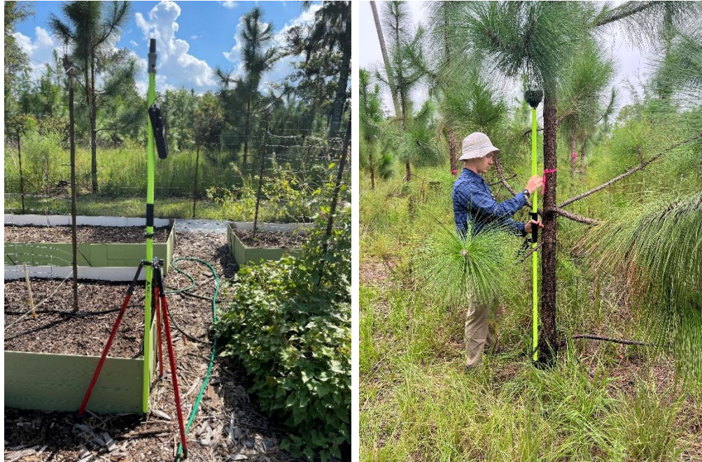
Figure 12. The GNSS base station (left) and rover (right) being used to record individual tree coordinates in September 2022. Right image courtesy of Dr. Thomas Jordan.
