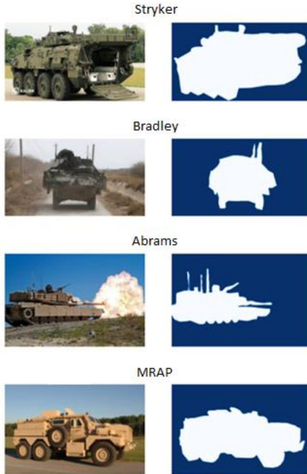
Figure 10: Manual annotations generated using VGG Image Annotator tool.
