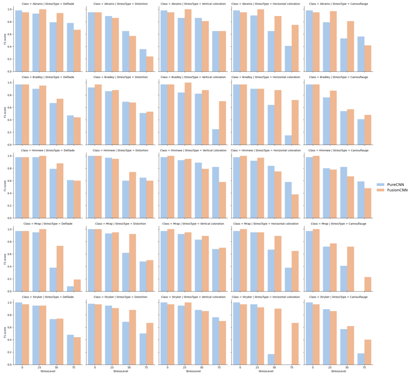
Figure 22: F1-score comparison (Resnet50 base). Top row to bottom row: target classes: Abrams , Bradley , HMMWW , MRAP , Stryker . Left column to right column: stressors: Defilade , Distortion , Vertical Coloration , Horizontal Coloration , Camouflage . X-axis: Stress levels (0%, 25%, 50%, 75%) . Y-axis: F1-score . Blue bar – PureCNN , Orange bar – CoNNText
