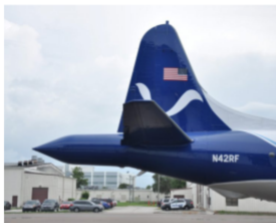
Figure 2: A current image of the TDR on the tail of NOAA's WP-3D N42 aircraft (Kermit). Source: AOML/NOAA
