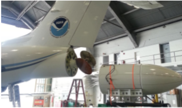
Figure 5: The dual-beam antenna of the TDR that's currently installed on NOAA's WP-3D and G-IV aircraft (as shown on the G-IV).
