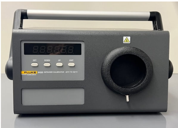
Fig. 2.2. Precision calibrator for thermal camera calibration.
