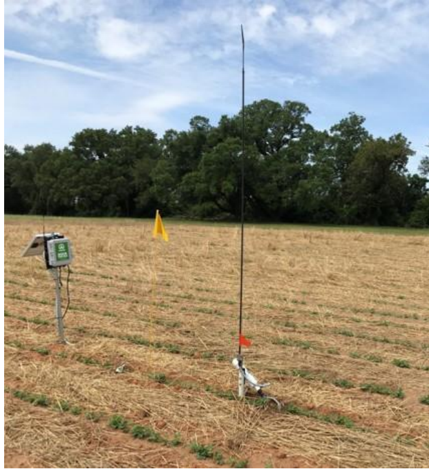
Figure 2.5. Plot 228-2 at the SIRP field during Year 1, where both Sentek probes with AGsense telemetry loggers (right) and UGA SSA sensors (right) were installed.
