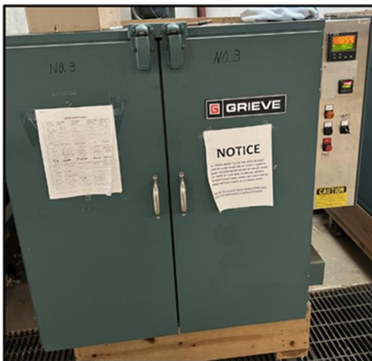
Figure 3: Heating oven, model: 13-261-28A (Grieve Corporation, Round Lake, Illinois, USA).
