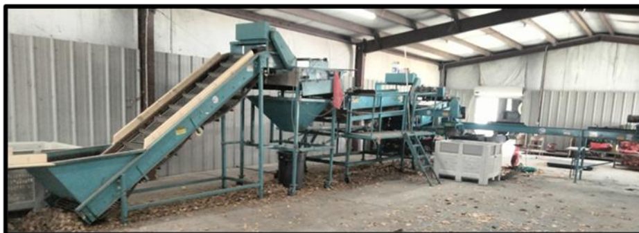
Figure 2: Onion grading machine (Haines Equipment Inc., New York, USA).
