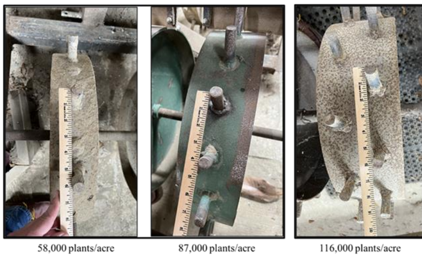
Figure 1: Equipment hole puncher types for different planting densities.
