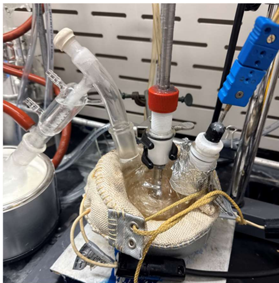
Figure 3.4. The reactor setup for polycondensation.
