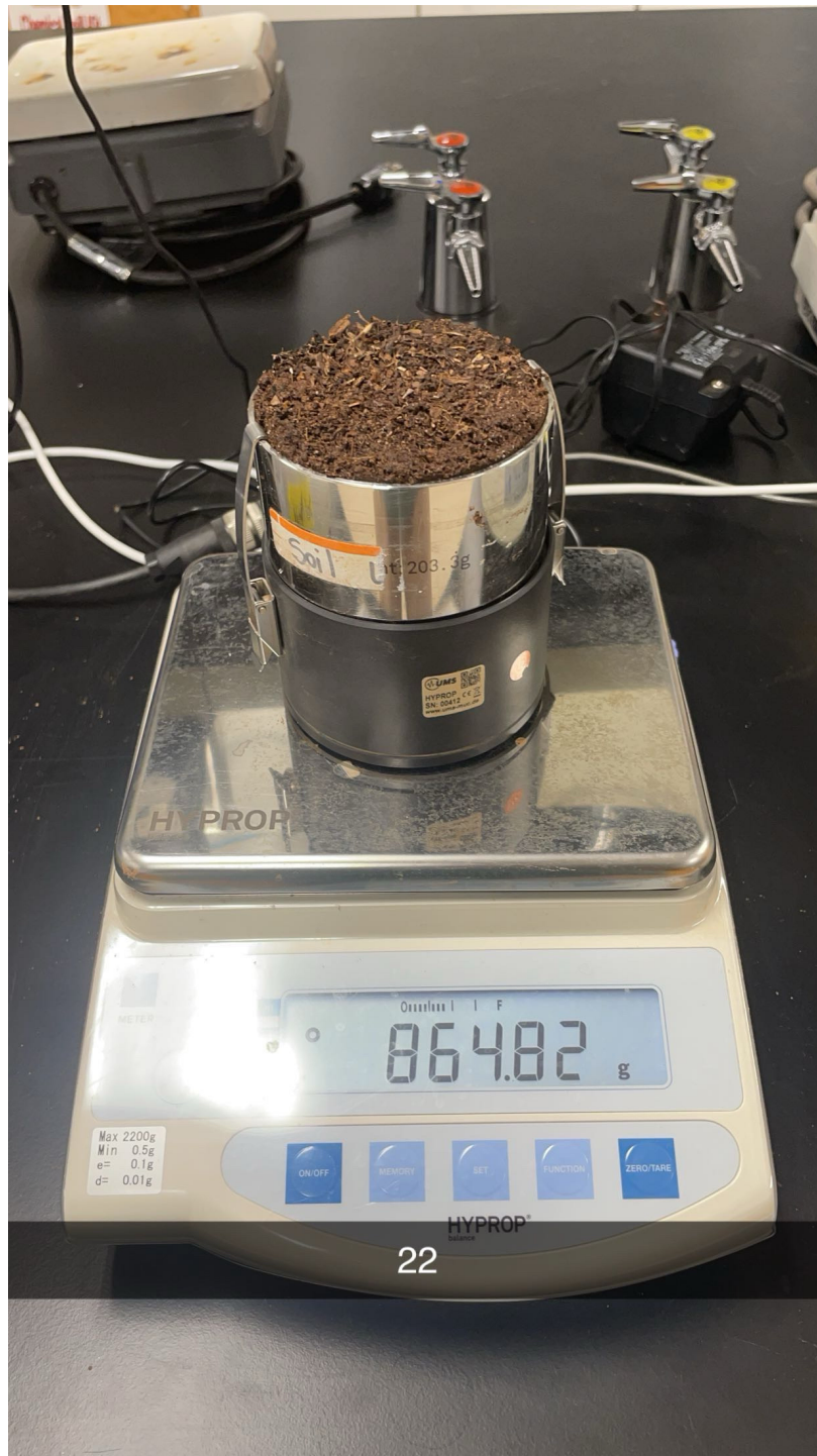
Figure 2.5: HYPROP setup that measures matric potential and volumetric water content simultaneously to obtain a soil moisture release curve.
