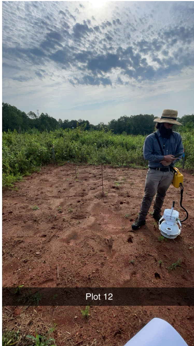
Figure 3.8: A picture of a disturbed plot a few days after the treatment. The picture captures soil respiration measurement using an automatic gas analyzer.
