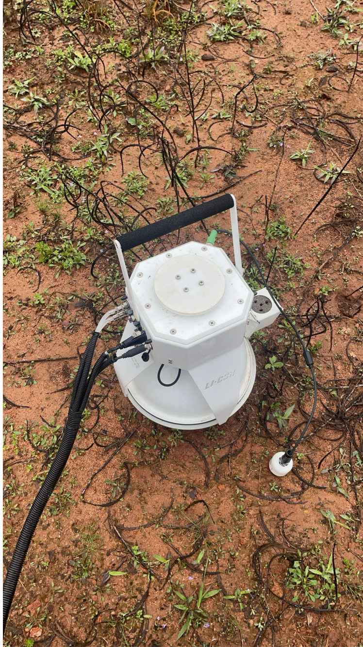
Figure 3.9: Automatic Gas Analyzer (LI-800, LI-COR®, USA), with an attached HydraProbe that measures soil water content and soil temperature.
