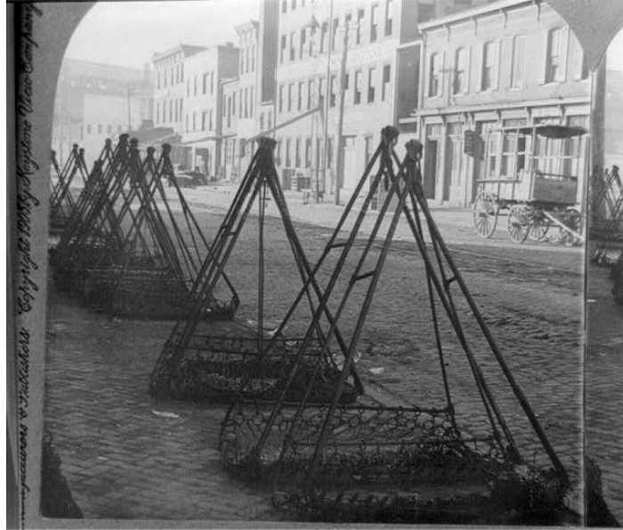
Figure 26. Metal oyster dredgers used to harvest oysters via sailboat lined up in the street in Baltimore, Maryland in the early 20 th century. From Dredgers (ca. 1905).
