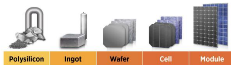
Figure 9: Solar PV Supply Chain [15].
