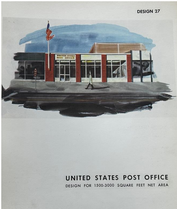
Figure 55: Thousand Series design drawing from Building Design Guidelines. Design 27 has an emphasis on horizontal bays split up by brick veneer with tall tri-part horizontal picture windows and silver window paneling (USPS Corporate Library, 1959).
