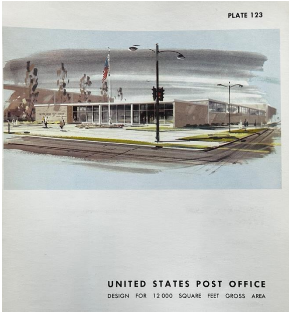
Figure 60: Thousand Series design drawing from Building Design Guidelines. Design 123 is a minimal design with no ornamentation other than the color, brick bond pattern, and vertical picture windows (USPS Corporate Library, 1959).
