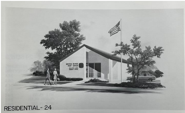
Figure 65: Thousand Series design drawing from Family of Standard Designs. Residential design 24 is a minimal design similar to design plate 54 from Building Designs. This post office also has a front gabled roof with recessed windows and an entrance. Construction materials were not specified in the guidelines (USPS Corporate Library, 1983).
