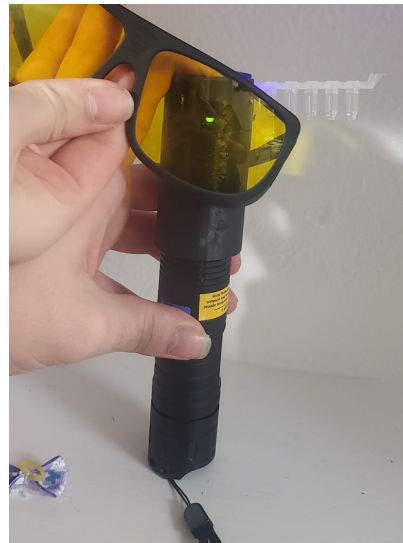
The results are viewed by shining the blue light on the tubes and viewing the samples through the blue light filtering glasses
