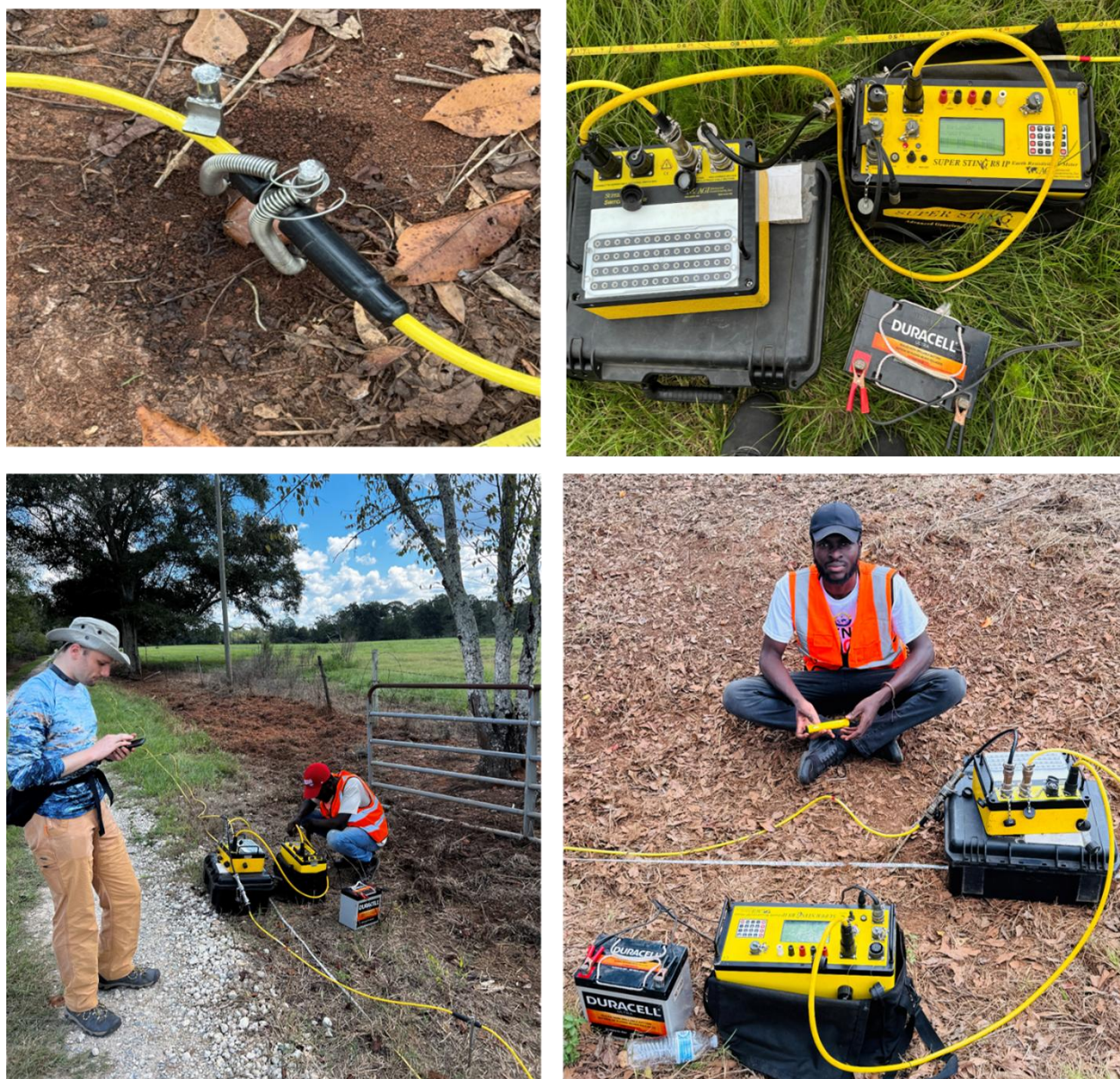
Figure 3.3: AGI Supersting R8 resistivity meter deployed in the field.
