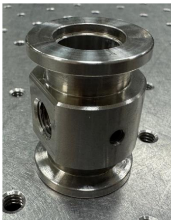
Figure 3.2.2 Custom NW16 extension with 1/16" drill tap.
