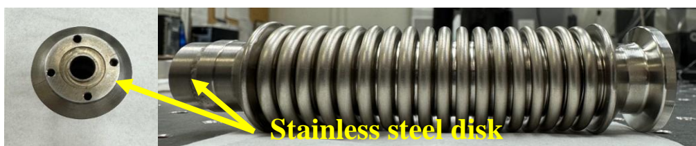
Figure 3.2.3 Custom bellow welded to stainless steel disk.
