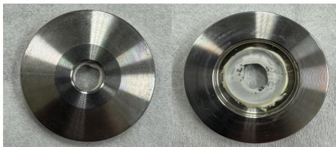
Figure 3.2.1 Front and back view of glued in CaF 2 window.
