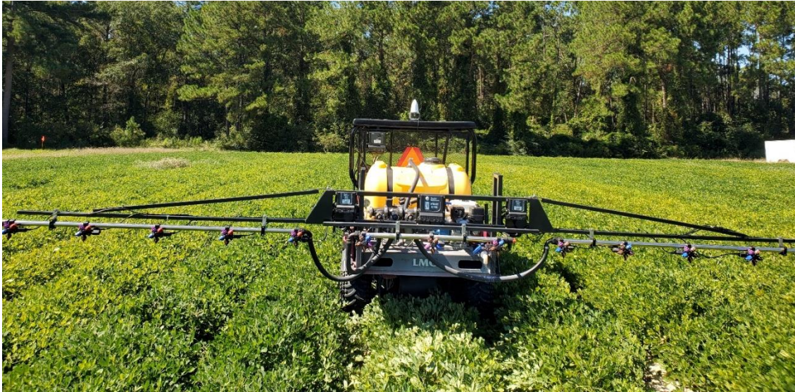
Figure 4.1 The 6-row UTV boom sprayer used for making fungicide applications and spray assessment in the field studies conducted in 2021 and 2022.
