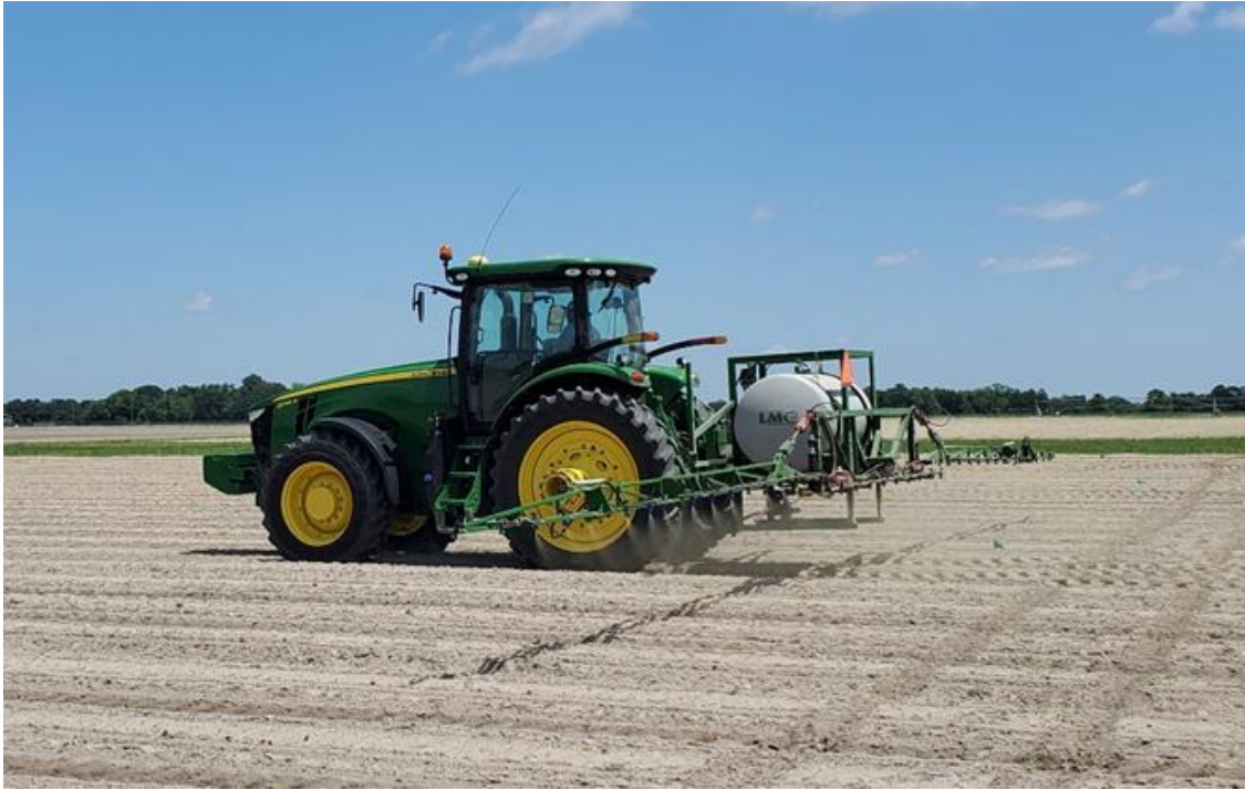
Figure 3.1 The commercial LMC boom sprayer used for making herbicide applications and spray assessment in the field studies conducted in 2021 and 2022
