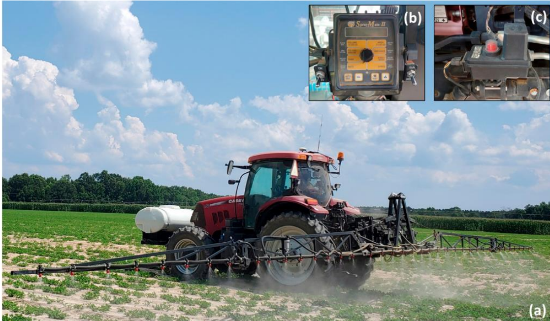
Figure 2.1 (a) The commercial Demco X-fold boom sprayer used for spray performance testing in 2021 and 2022. (b) The Micro-Trak MT-2405F II rate controller and (c) the TeeJet® 346BPR-2F-03 regulating valve used in 2022.
