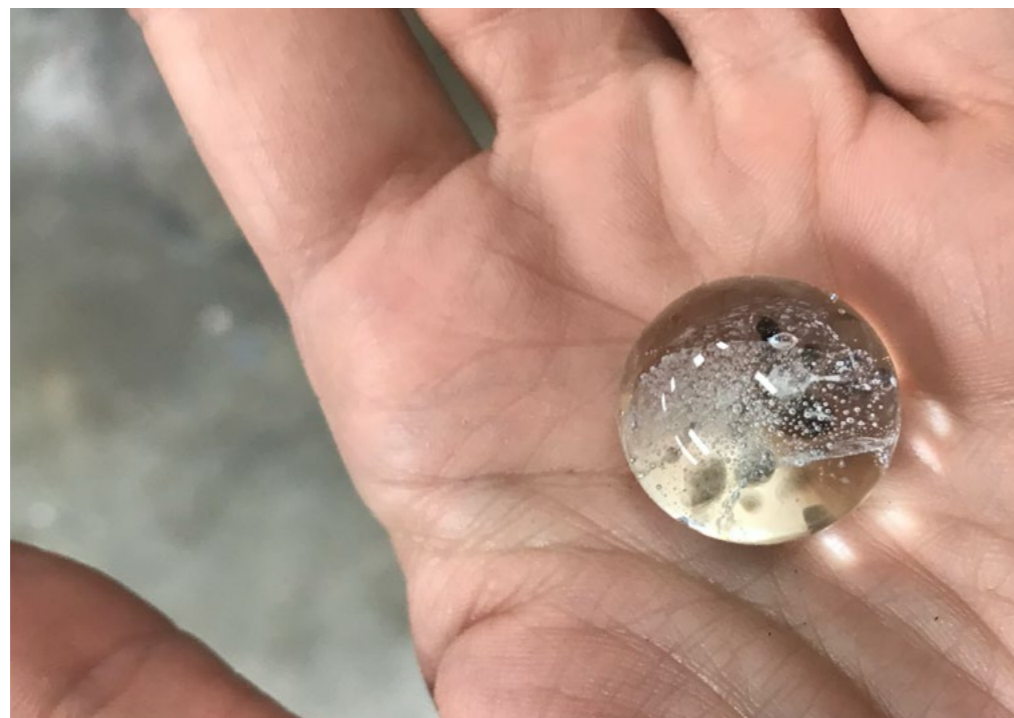
Fig. 24 Glass marble with ash inclusions, fabricated by Annalee Pickett, University of Georgia Scientific Glass Blowing Shop
