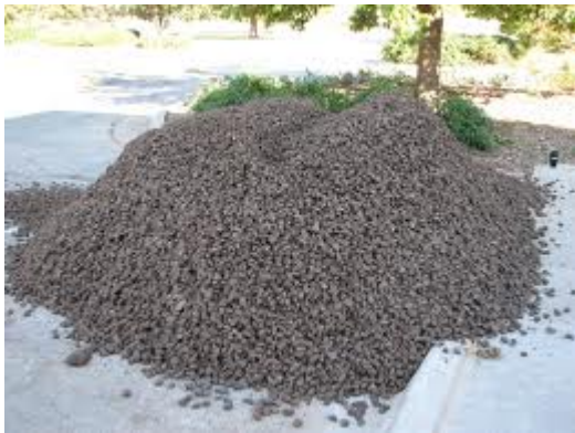
Figure 4.1. Image of CU-Soil demonstrating large aggregate structure. Photo courtesy of JV Environmental, Austin, TX.
