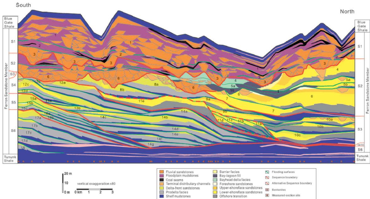
FIG. 15.—Dip stratigraphy of the Ferron Notom Delta. Forty-three parasequences have been identified. They are further grouped into 18 parasequence sets. Five sequence boundaries are recognized, and six depositional sequences (S1-S6) are defined. See detailed correlation panel with measured sections in the JSR data archive, see Acknowledgments section.
