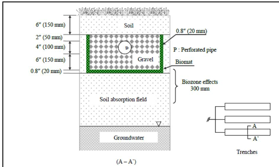
Figure 2.2. Configuration of a septic tank effluent distribution chamber and absorption system showing the formation of the biozone layer (Neitsch et al., 2011).
