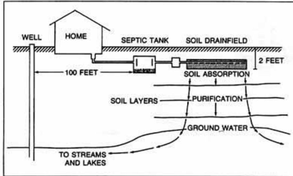
Figure 2.1. Diagram of a conventional on-site wastewater treatment system. Domestic wastewater enters from the house, undergoes physical, chemical and biological processes, and then is released to the drainfield for further purification (Jones and Yahner, 2008).
