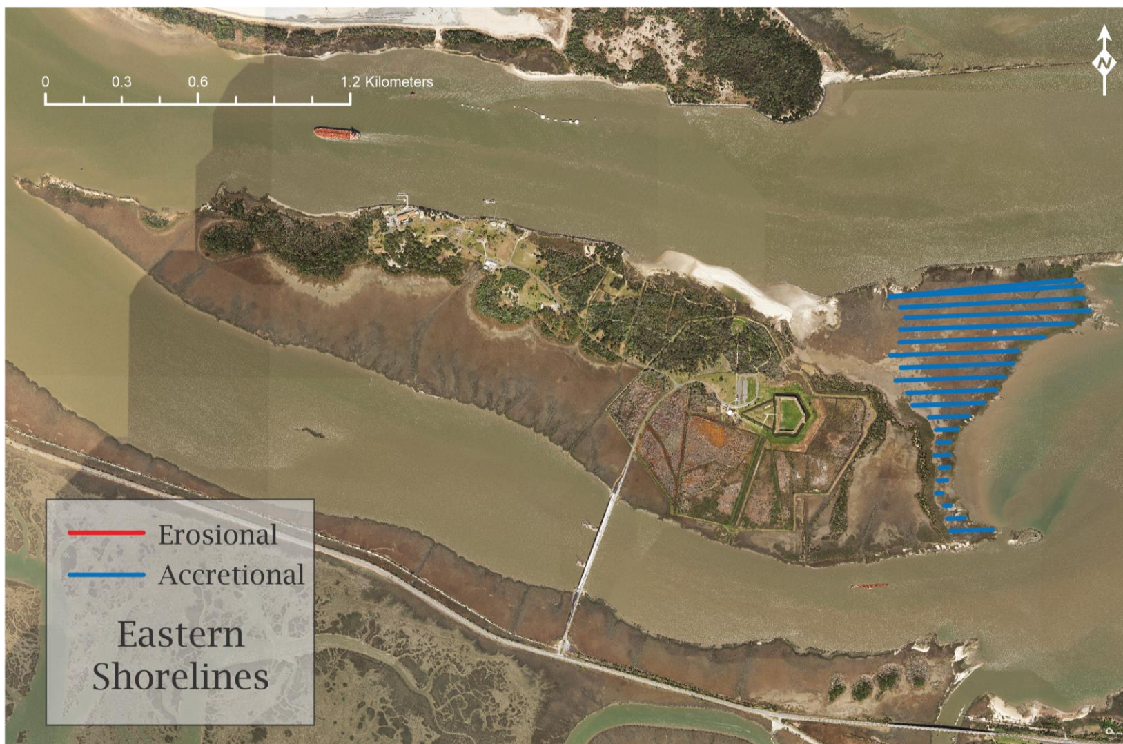
Figure 8. AMBUR produced transects of Cockspur Island eastern shoreline. Length of transects represent the magnitude of change. Analysis performed with all shoreline transects, from 1933 to 2018. Blue transects indicate net accretion, there are no erosional transects.
