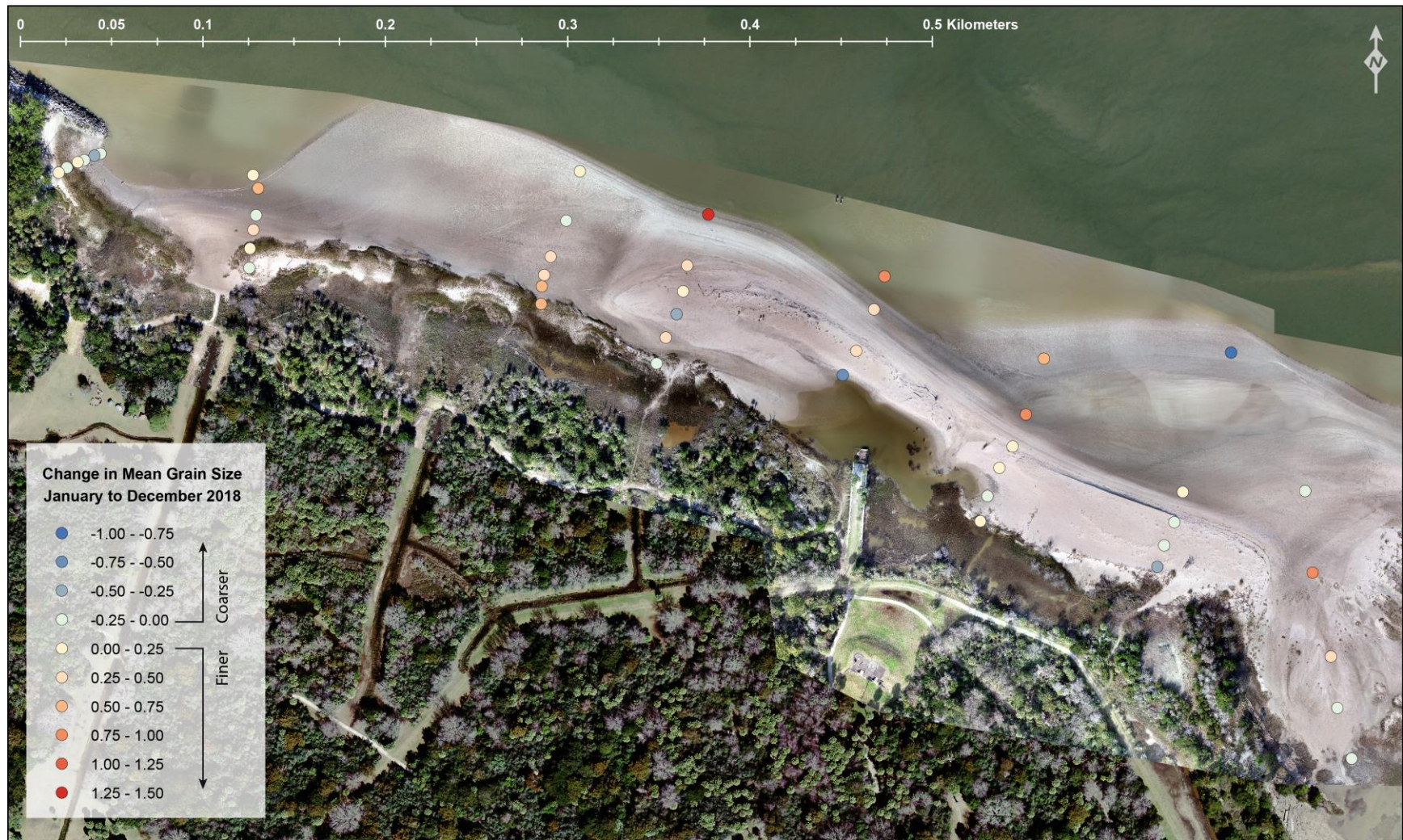
Figure 33. Map of change in Mean Grain Size, in phi, on Cockspur Island, on the nourished northern shoreline. Cool colors indicate mean grain size becoming finer, warm colors indicate mean grain size becoming coarser.
