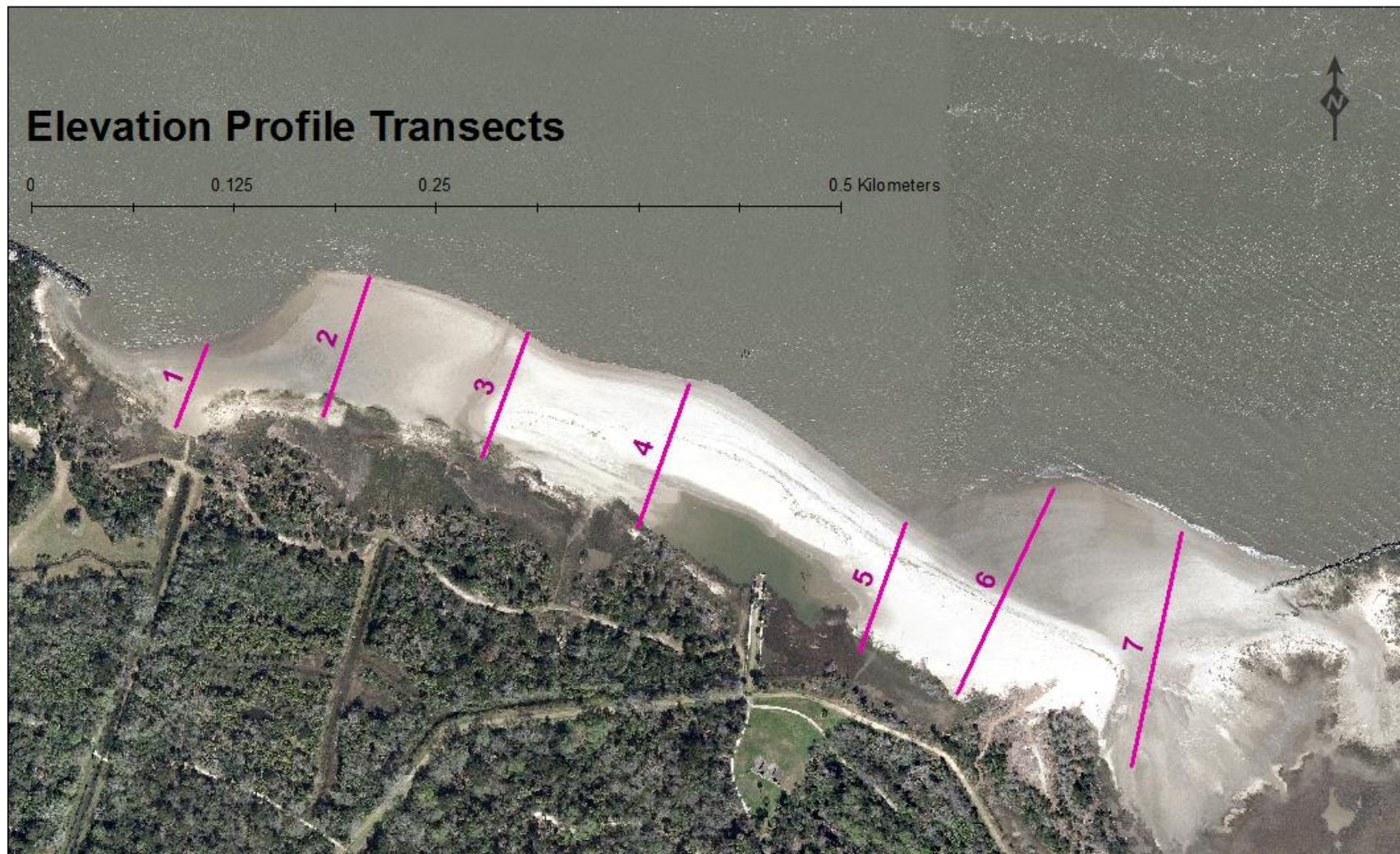
Figure 20. Map of transect locations for elevation profile comparisons on Cockspur Island's nourished northern shoreline. Transects are labeled from the western end to the eastern end of the shoreline. Transects are measured from the channelward edge to the landward edge.
