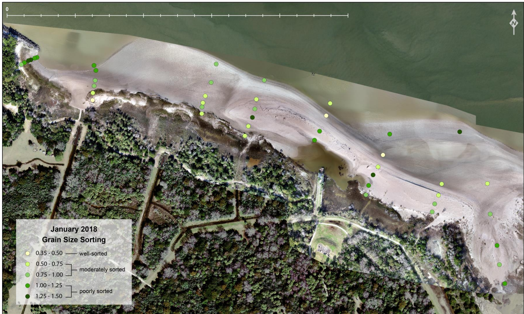
Figure 29. Map of grain size sorting of the nourished northern shoreline on Cockspur Island, for January 2018. Light hues indicate poorer sediment grain size sorting; darker hues indicate more well-sorted sediment grain size
