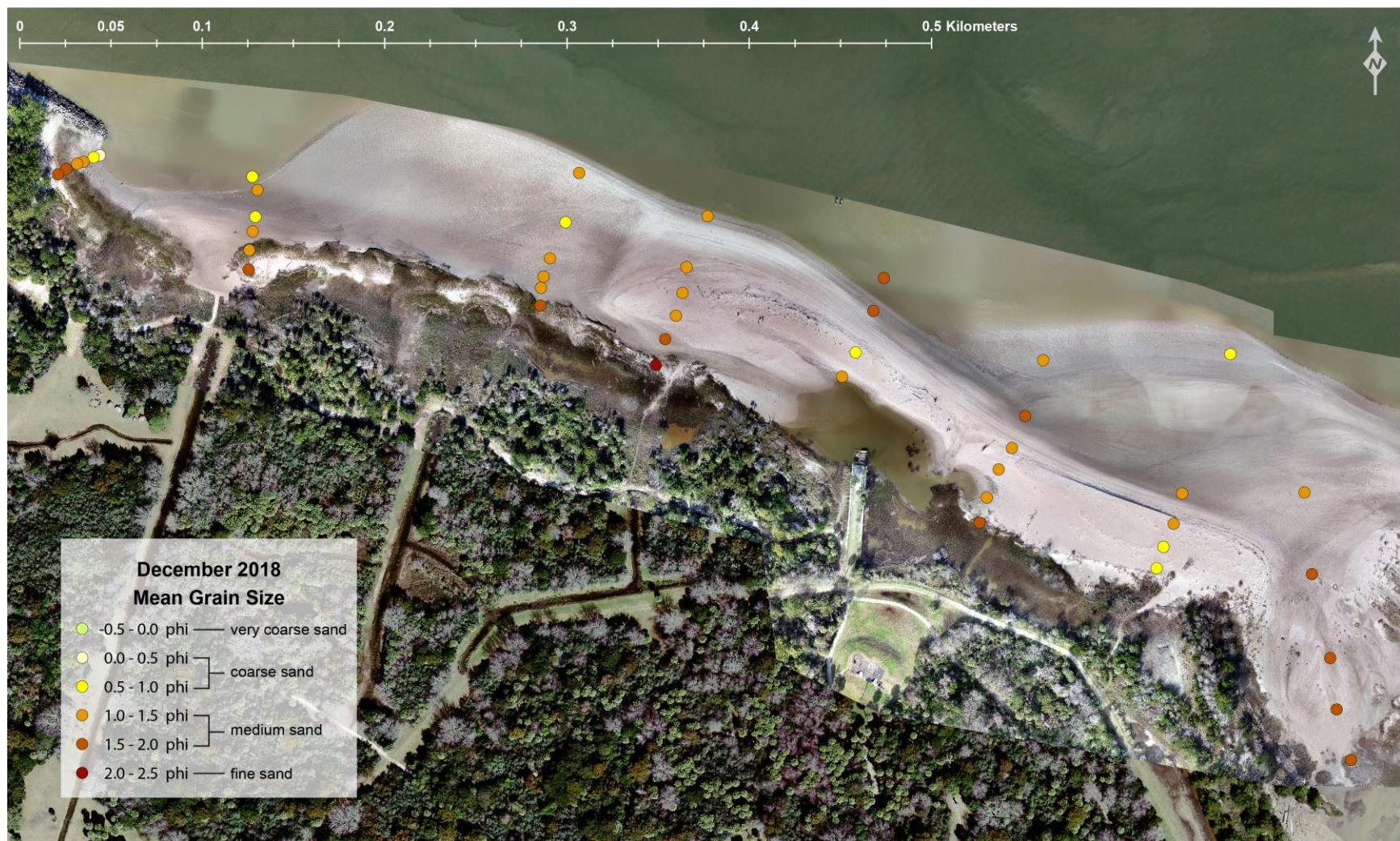
Figure 30. Map of mean grain size, in phi, of the nourished northern shoreline on Cockspur Island, for December 2018. Light hues indicate finer sediment grain size; darker hues indicate coarser sediment grain size.
