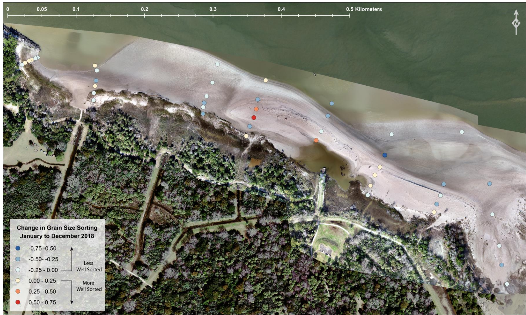
Figure 34. Map of change in Grain Size Sorting on Cockspur Island, on the nourished northern shoreline. Cool colors indicate grain size becoming less well-sorted, warm colors indicate grain size becoming more well-sorted.
