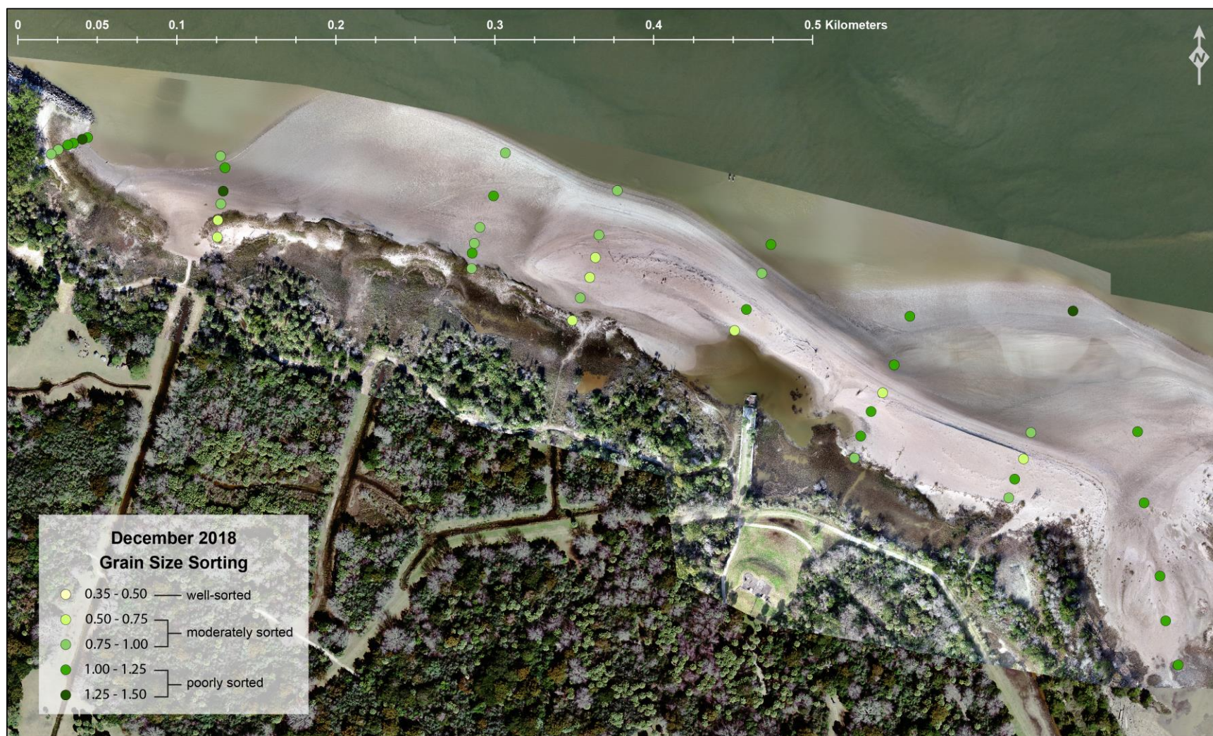
Figure 31. Map of grain size sorting of the nourished northern shoreline on Cockspur Island, for December 2018. Light hues indicate poorer sediment grain size sorting; darker hues indicate more well-sorted sediment grain size.
