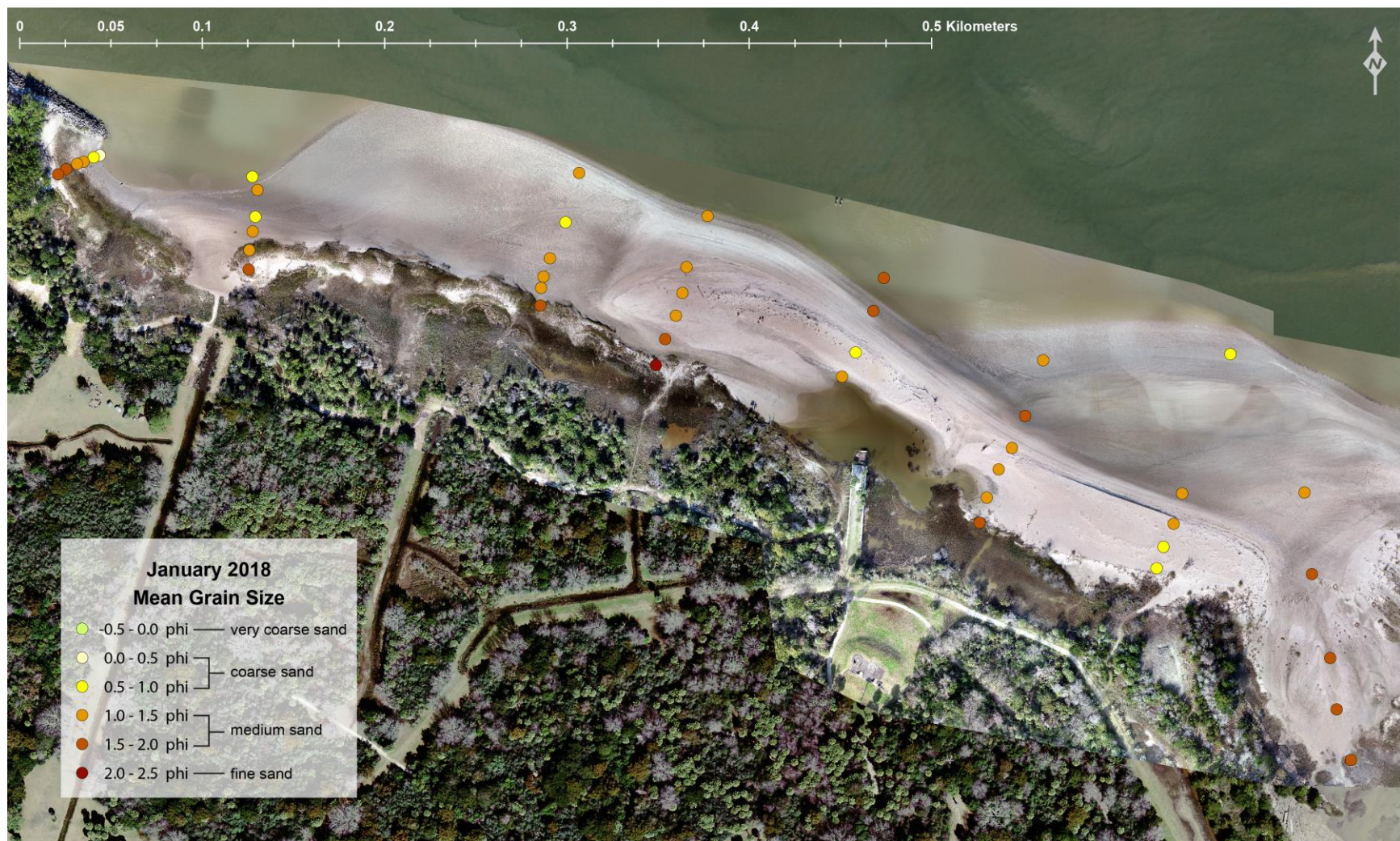
Figure 28. Map of mean grain size, in phi, of the nourished northern shoreline on Cockspur Island, for January 2018. Light hues indicate finer sediment grain size; darker hues indicate coarser sediment grain size.
