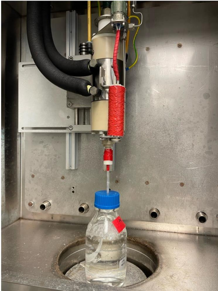
**Figure. 3.1** Cold plasma treatment of potable water (PW) using the DBD plasma.
