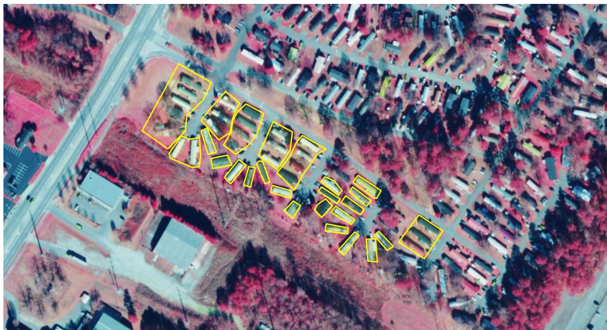
Figure 12- Examples of polygons drawn around mobile homes for training samples.
