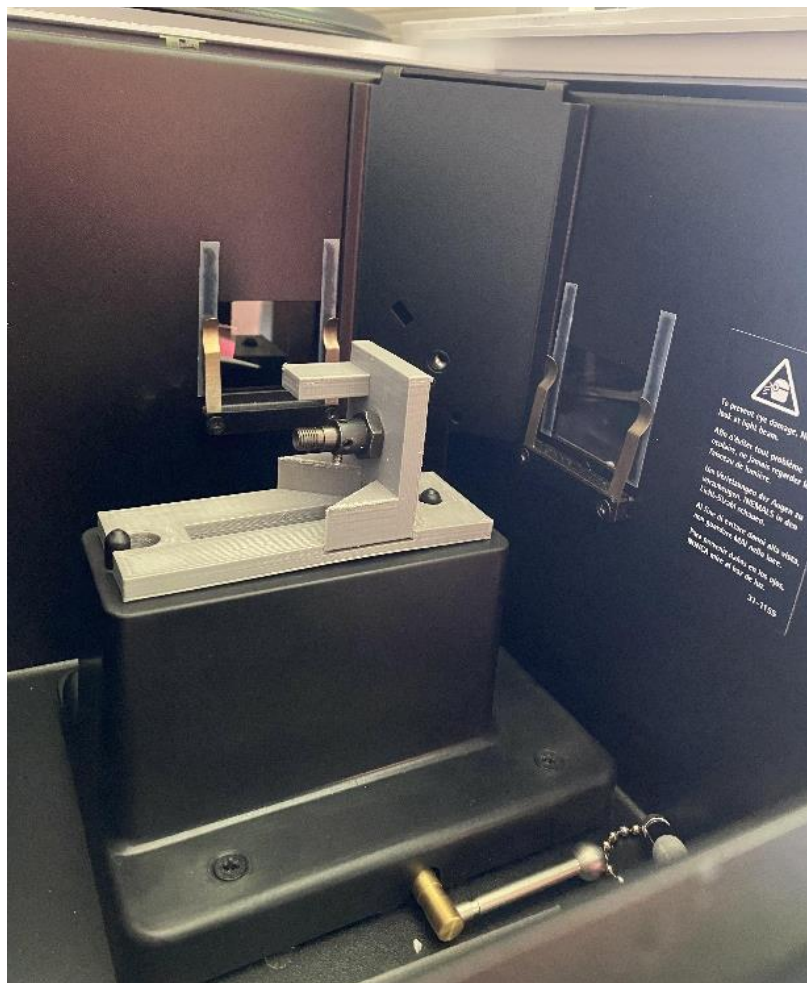
Figure 3.4. Cary Eclipse Fluorescence Spectrophotometer base with 3D printed fiber optic attachment
