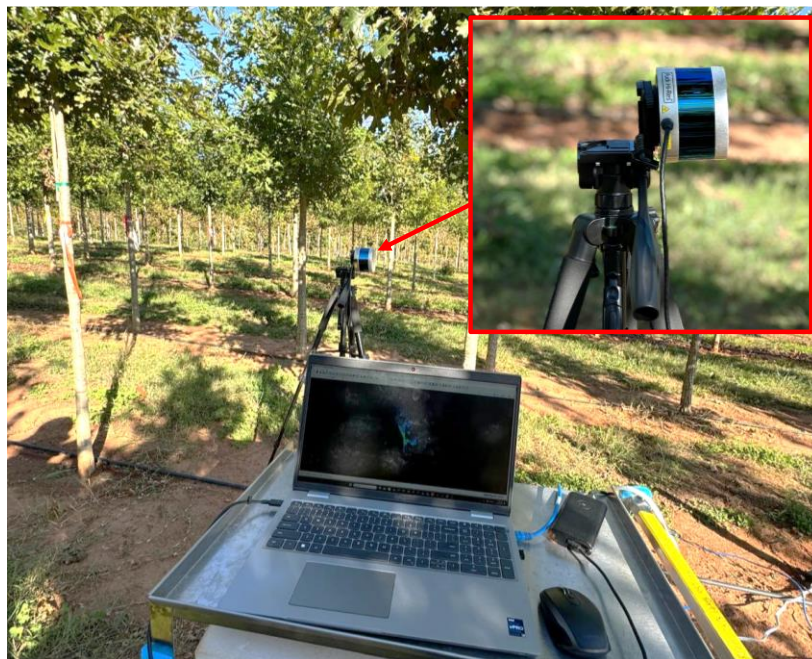
Figure 4.3. LiDAR system setup for tree canopy data collection, featuring a Velodyne VLP-16 LiDAR sensor mounted on a tripod for stable positioning. A laptop, placed on a mobile lab workstation, is used for recording and visualizing the LiDAR data streams in real-time.
