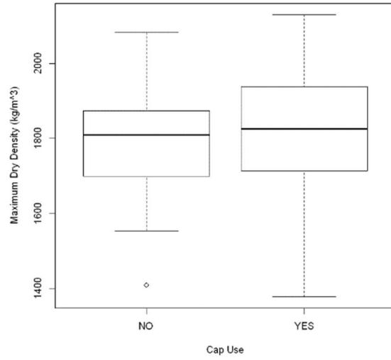
*Figure B-12: Maximum dry density versus use of caps*
