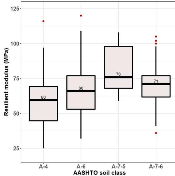
*Figure 5-8:  $M_R$  ranges for AASHTO soil classes (testing dataset)*
