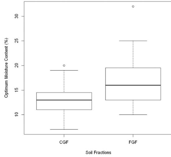
*Figure C-26: Optimum moisture contents versus non-granular soil fractions*
