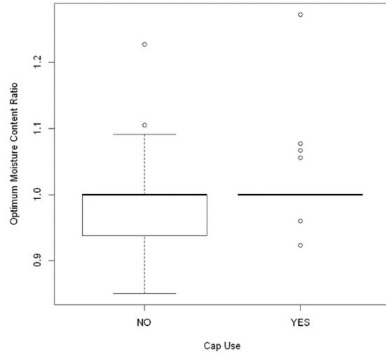
*Figure D-38: OMC ratios of the fine-grained soil fraction versus use of caps*
