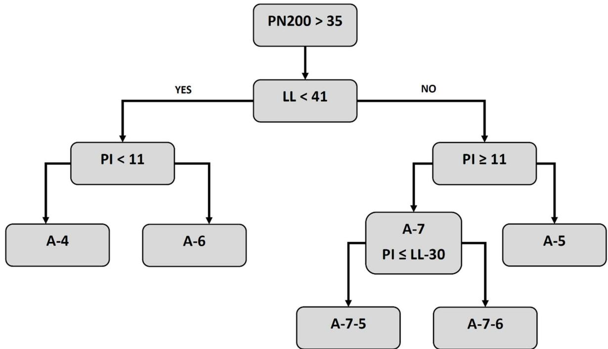
*Figure 3-2: AASHTO M-145 for non-granular soils in a decision tree format*
