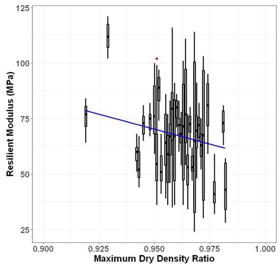
*Figure 4-26:  $M_R$  vs Compaction*
