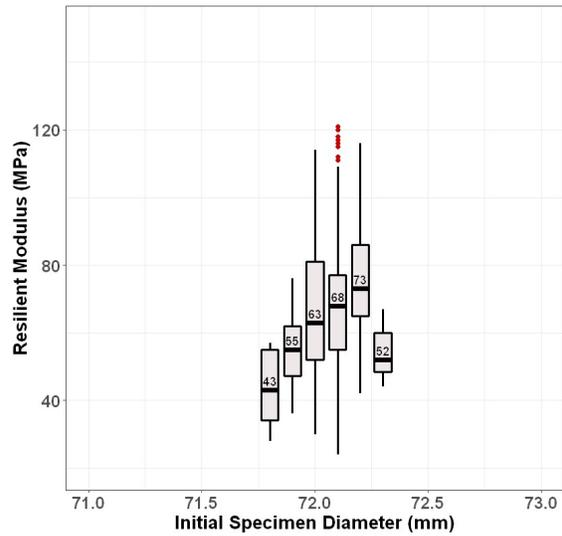
*Figure 4-17:  $M_R$  vs Initial Diameters*
