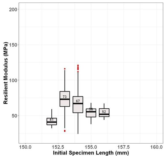
*Figure 4-18:  $M_R$  vs Initial Lengths*
