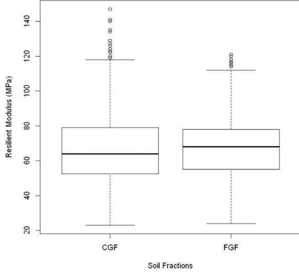
*Figure C-20:  $M_R$  versus soil fractions*
