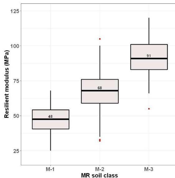
**Figure 5-7:  $M_R$  ranges for M classes (testing dataset)**
