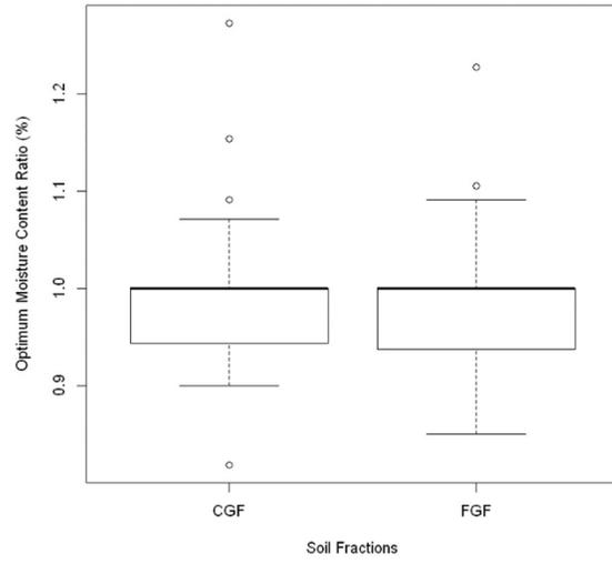
*Figure C-28: Optimum moisture content ratios versus non-granular soil fractions*
