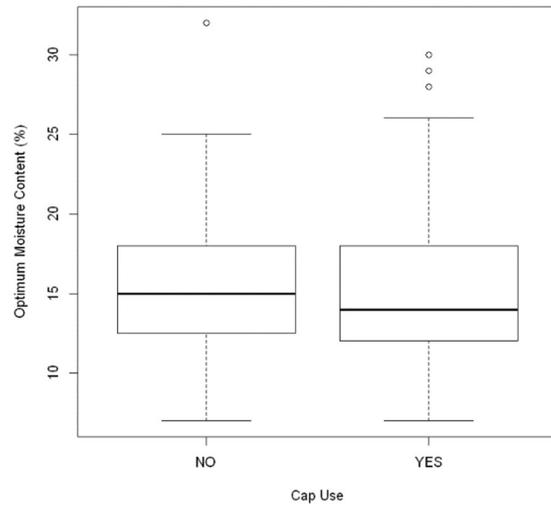
*Figure B-16: Optimum moisture content versus use of caps*
