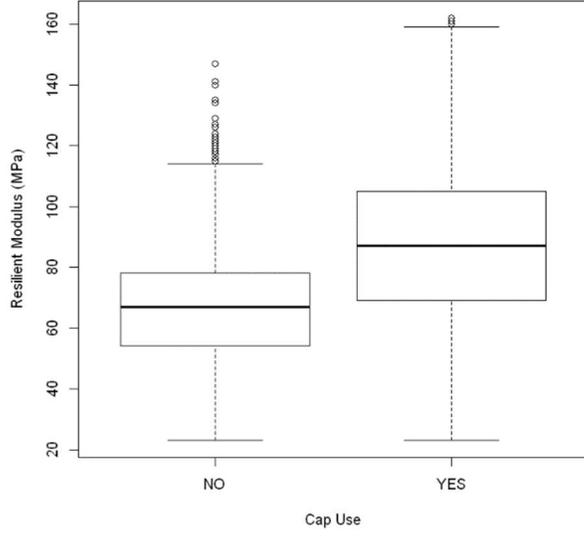
*Figure B-10:  $M_R$  versus use of test caps*
