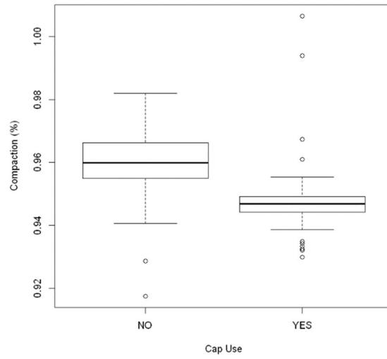
*Figure D-34: Compaction of the fine-grained soil fraction versus use of caps*
