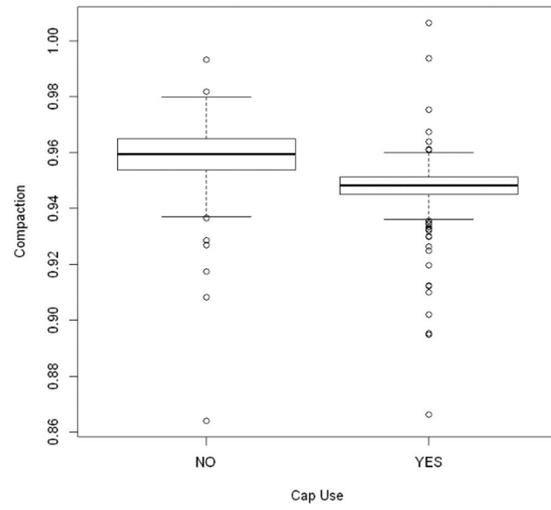
*Figure B-14: Compaction versus use of test caps*
