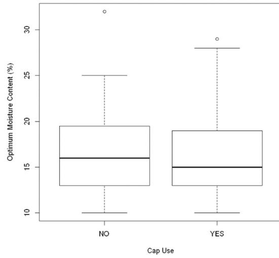
*Figure D-36: OMC of FGF versus the use of caps*
