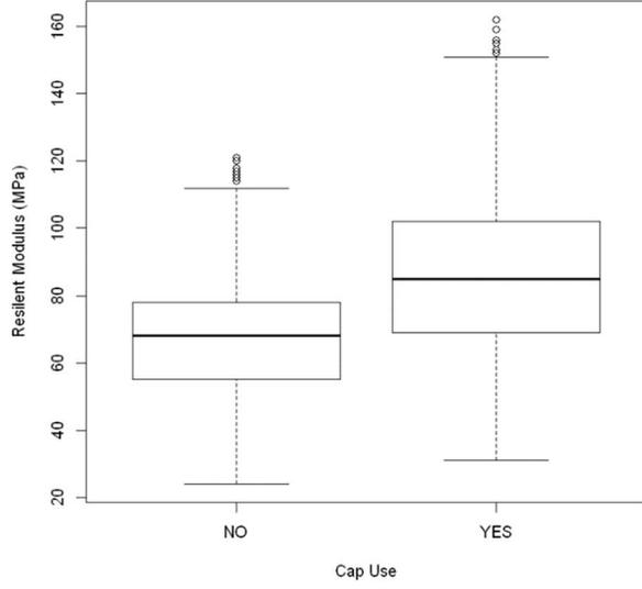
*Figure D-30:  $M_R$  of the fine-grained soil fraction versus use of caps*
