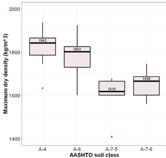
*Figure 4-15: Maximum dry density by AASHTO class for FG soils*
