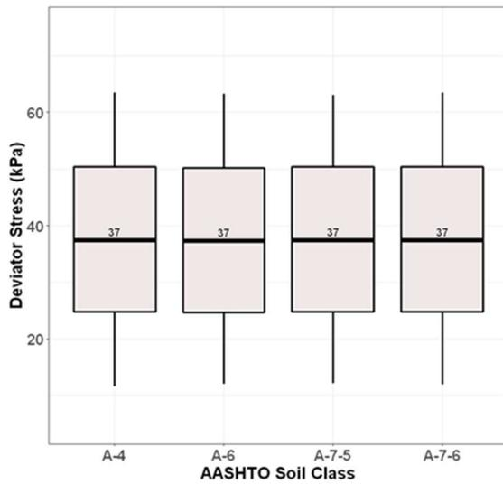
*Figure 4-13: Deviator stress by AASHTO class for FG soils*
