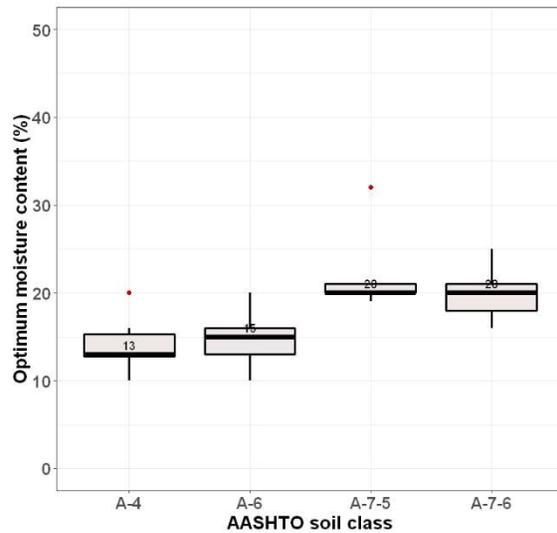
*Figure 4-16: Optimum moisture content by AASHTO classes for FG soils*
