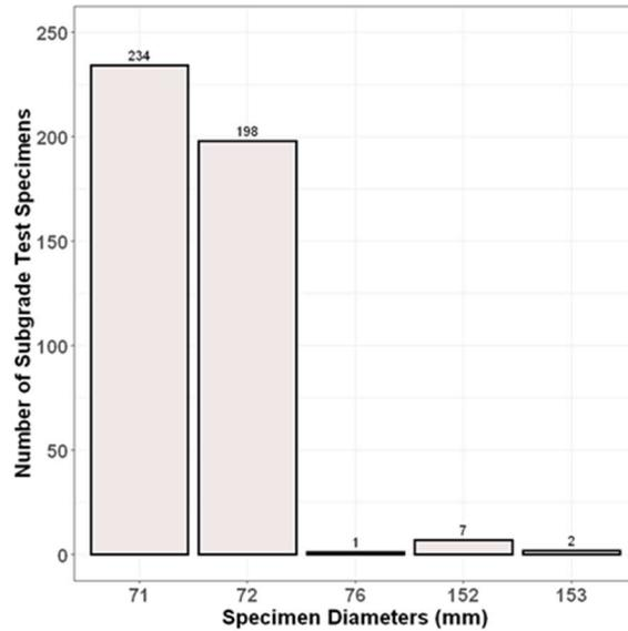
Figure 4-2: Distribution of specimens in the raw dataset by mold diameter
