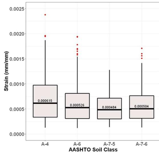
*Figure 4-14: Strain by AASHTO class for FG soils*
