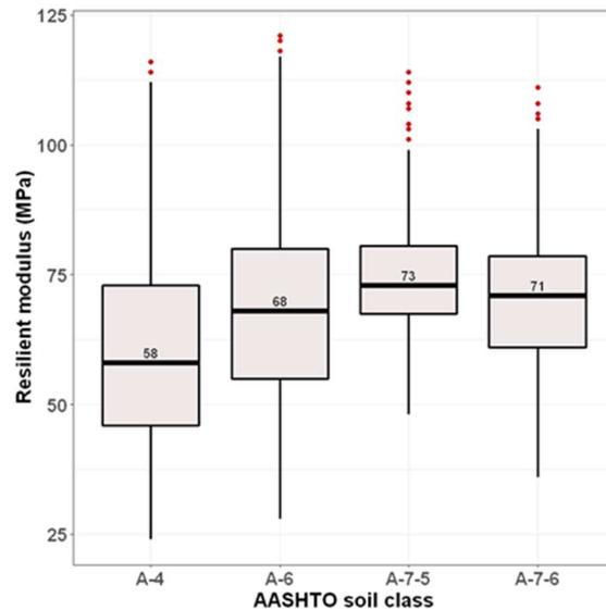
*Figure 4-12:  $M_R$  ranges by AASHTO soil classes (FG soils)*
