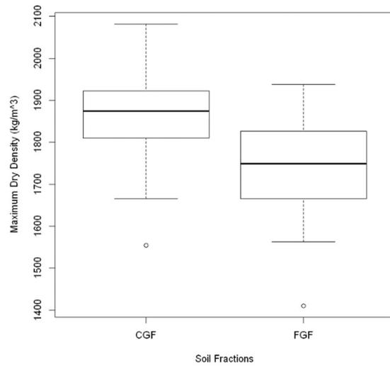
*Figure C-22: labMDD versus non-granular soil fractions*
