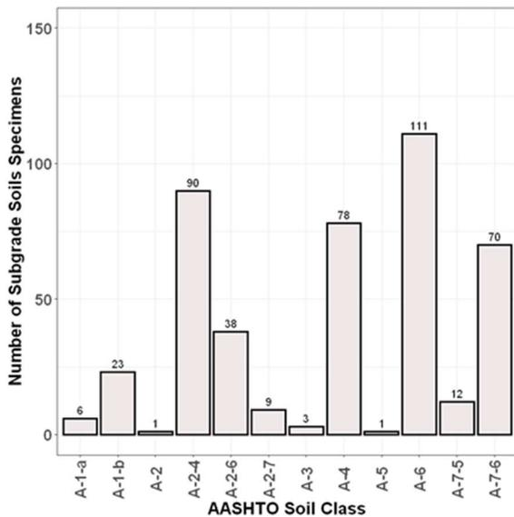
Figure 4-3: Granular and non-granular specimens by AASHTO soil class
