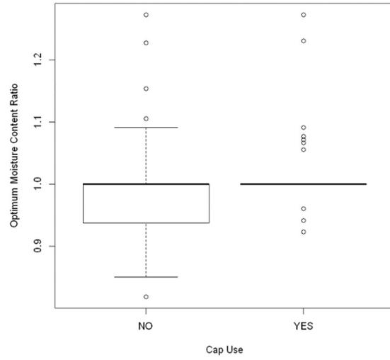
*Figure B-18: Optimum moisture content ratios versus use of test caps*
