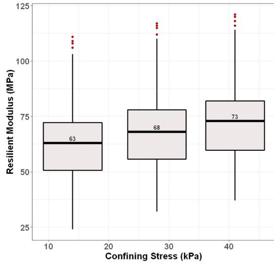
*Figure 4-21:  $M_R$  vs confining stress*
