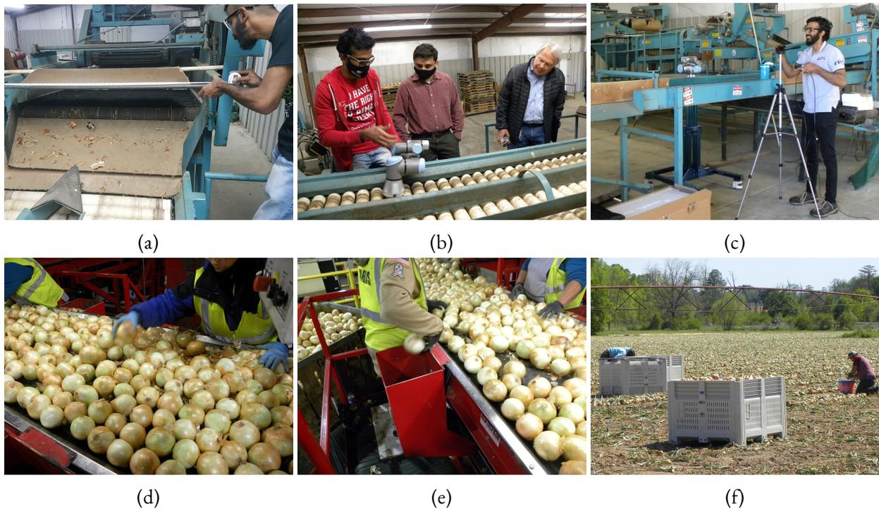
Figure 1.6: (a) Collecting measurements of the conveyor system at VOVRC to build the cobot environment appropriately. (b) Brainstorming ideas on how the cobot could be deployed as a turnkey solution that leaves the existing conveyor system undisturbed. (c) Setting up our cobot and its camera feed for demo and testing. (d – f) Field research conducted at multiple sorting sheds and farms to gather information about human workers and their existing sorting procedures.
