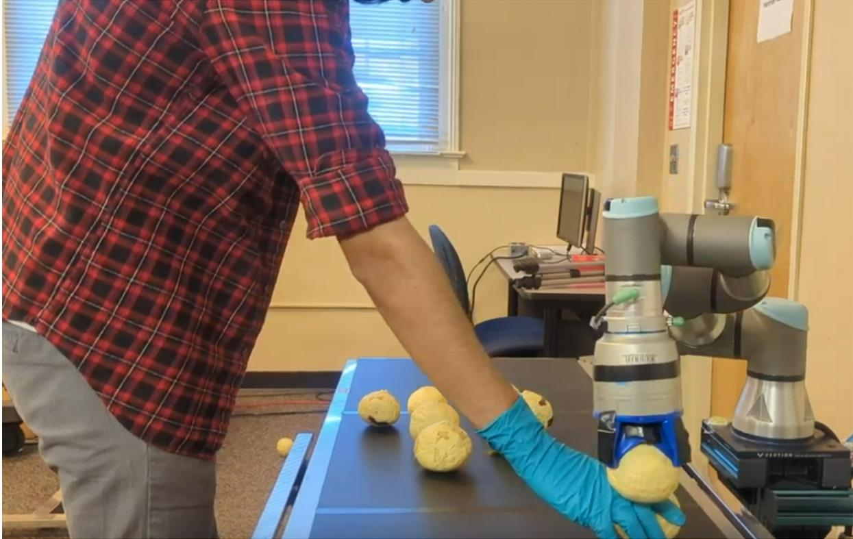
Figure A.9: Figure shows a cobot colliding with human after they entered the workspace during cobot trajectory.
