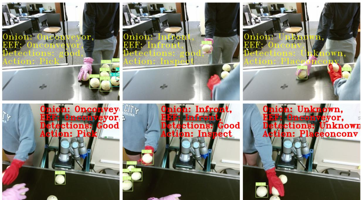
Figure 6.5: Image frames from a data set used to obtain the joint state-action trajectories  $\mathcal{X}^E$  via SA-Net (Soans et al., 2020). The annotations on the images are the state-action predictions and the bounding boxes are generated by YOLOv5. The first frame is when the onion is on the conveyor and the human expert is about to pick. The second is when the human is inspecting and finding a good onion. The third is when the human is placing the onion back on the conveyor.
