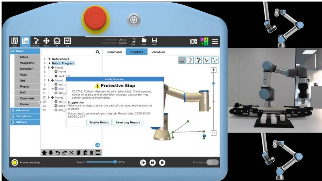
Figure A.6: Figure shows the protective stop occurring on a Universal Robots cobot while manipulating objects. Image credit: Universal Robots
