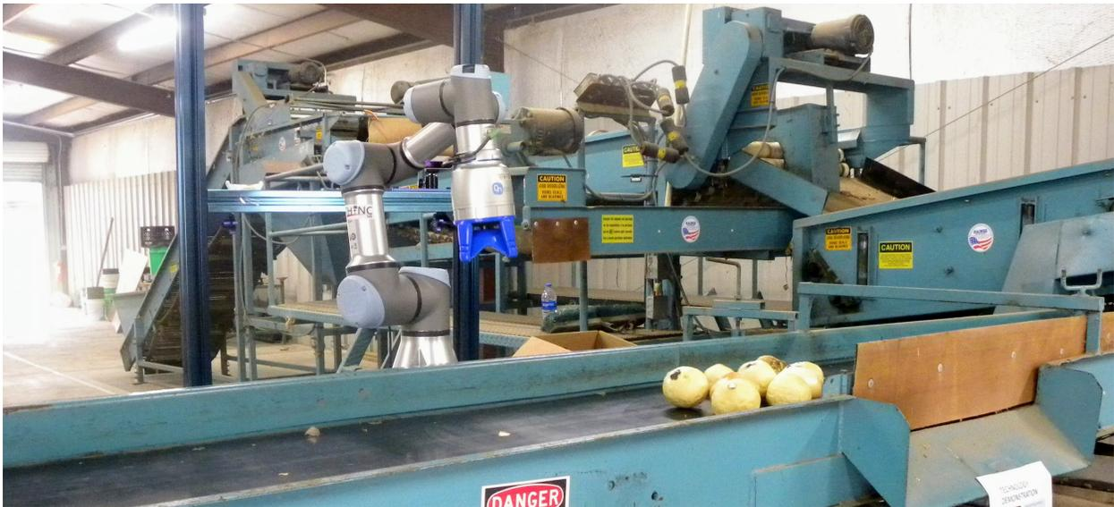
Figure A.1: Cobot UR3e deployed beside an industrial conveyor at a real-world onion sorting shed.
