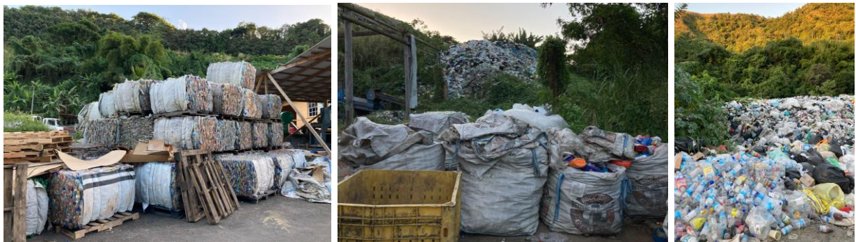
Figure 4.42: Field photos from the Fond Cole landfill, showing baled PET bottles and those waiting to be baled
