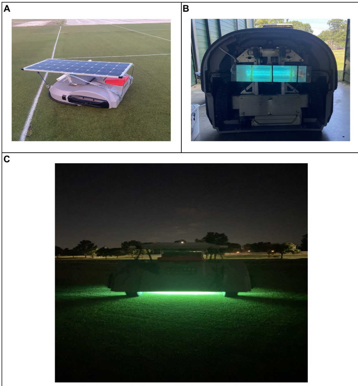
Figure S3.2: Modified Echo Robotics TM-1000 Turf Mower used to apply UV-C treatments in field trials (A). Panel B shows the UV-C light mounted to the bottom of the mower chassis, and Panel C shows nighttime operation in the field with the UV-C light powered on.
