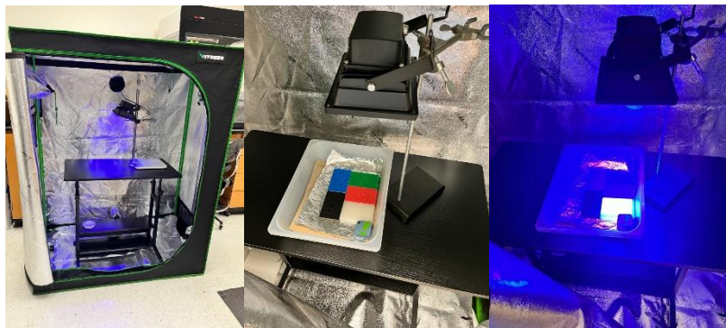
Figure 4.1: Pictorial representation of aBL set up used for the study. (a) aBL set up (b) HPDE coupons before treatment (c) HDPE coupons during Blue light treatment
