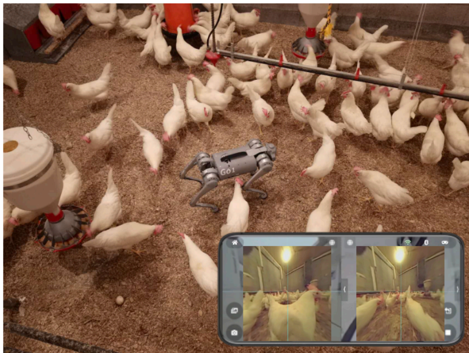
Figure 6.2. Overview of the automated detection system for poultry management using YOLOv8 and Unitree Go 1 Robotic.
