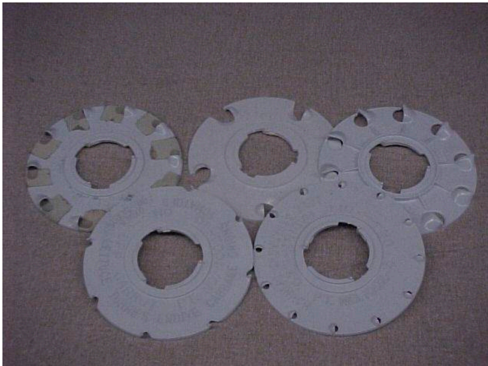
Figure 2. Various plates used the Earthway planter.
