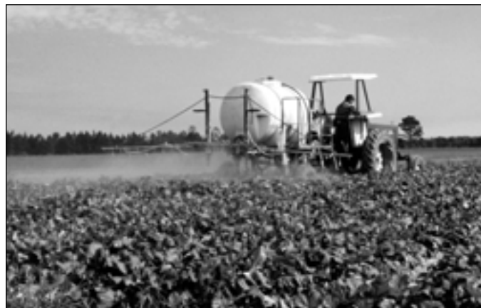
Figure 42. Hydraulic boom sprayer
