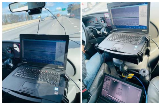
Figure 17 UGA GPR road survey control units
