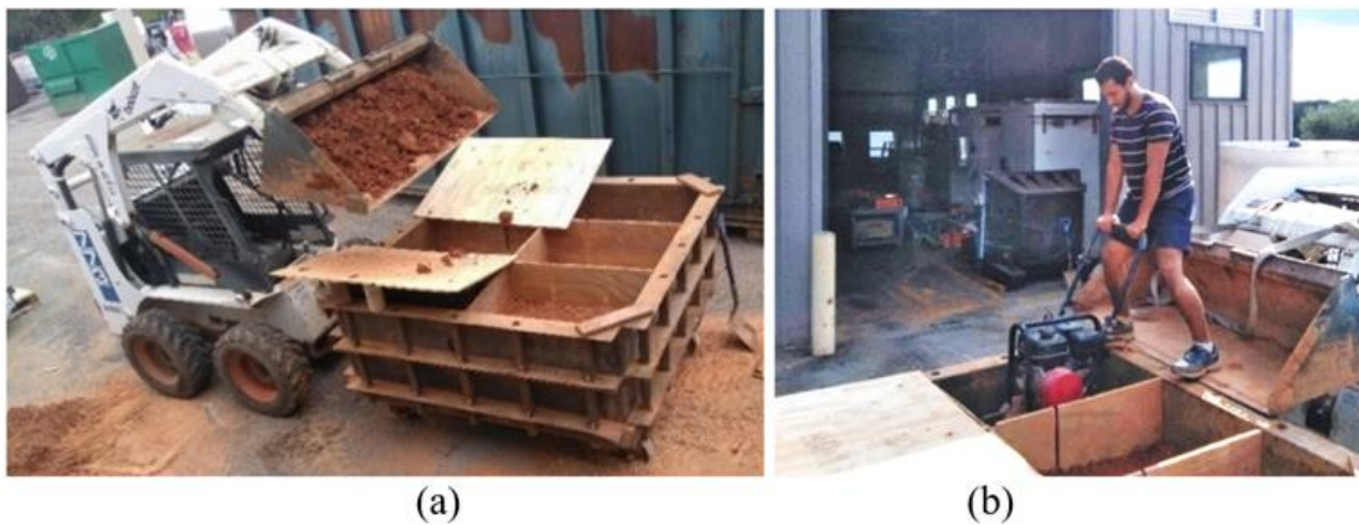
Figure 8 Sample preparation photos: (a) Soil transportation and filling testing box, (b) soil compaction
