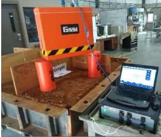
Figure 10 GPR Scanning and calibration for different samples
