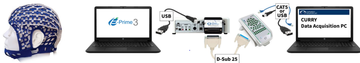
Figure 10 : EEG 32-channel Cap and Hardware Device [156]
