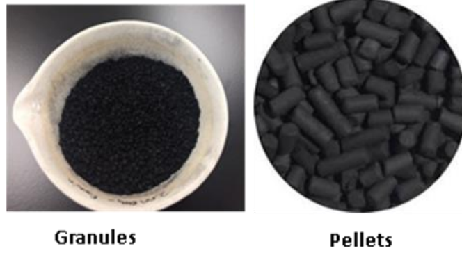
Figure 2.2. Activated carbon in the form of granules and pellets.
