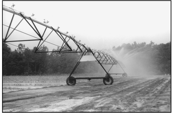
Figure 3. Center pivot irrigation system with medium pressure impact sprinklers
