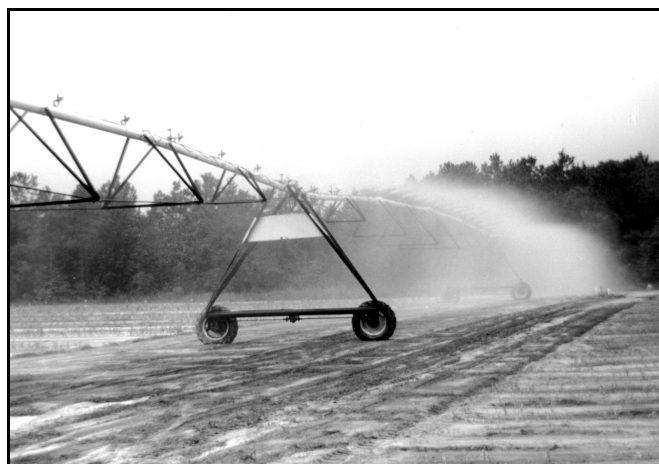
Figure 1. Center pivot irrigation system with low pressure spray nozzles.
