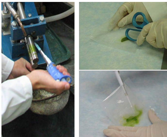
FIGURE 2. Plant sap being extracted by a leaf press (left) and the use of mesh bags (right).
