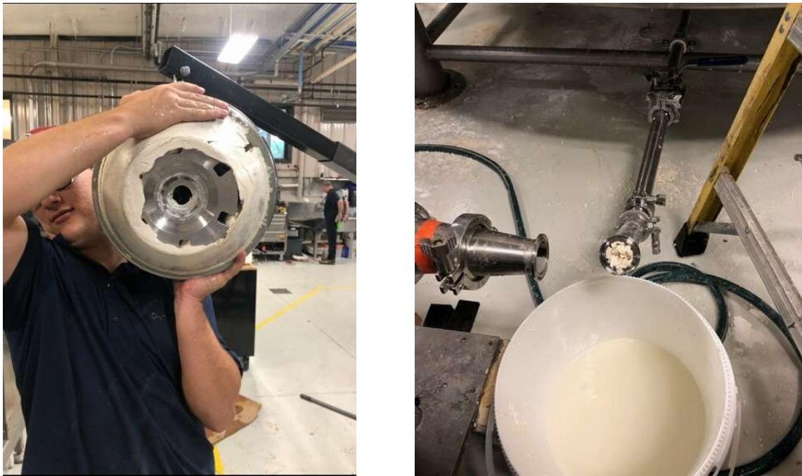
Figure 1.6: Left: Centrifuge operator displaying a seized disc-stack due to polymer crystallization during compaction. Right: Clogged pipe due to large agglomerates formed during separation in a decanter centrifuge. Image credit: Bryan Scott, RWDC Industries
