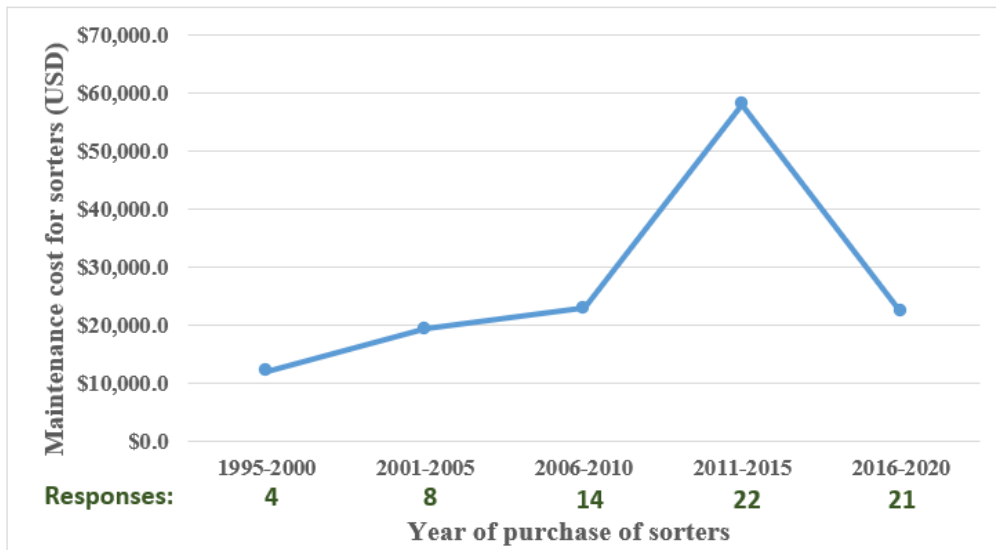
Figure 6.3: Maintenance cost vs. year of purchase of (A) analyzers and (B) sorters. All monetary data has been converted to US currency to facilitate comparisons between countries. Overall, the newest analyzers and sorters costed more in maintenance as compared to oldest analyzers and sorters.
