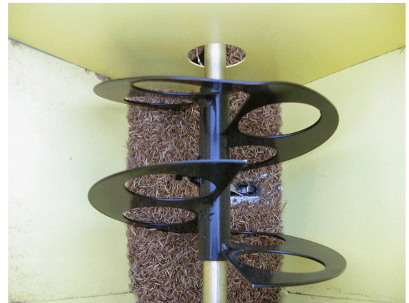
Figure 9. A seed box agitator is necessary to prevent the fluffy seeds of some NWS grasses from clogging openings in the seed box.
