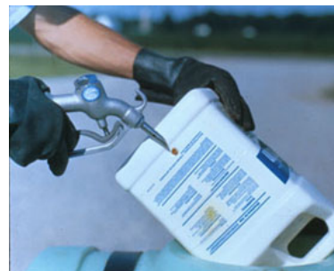
Figure 3. Tools can be purchased that will puncture and rinse chemical containers. Qwik-Rinse and Jet Rinse are two brand names. Photo courtesy Quik-Rinse, Inc.
