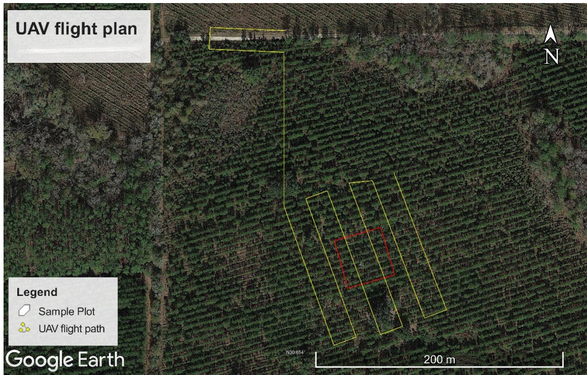
Figure 4.2 Figure shows the UAV-flight plan to collect lidar data, which was created in UGCS software and projected over google earth pro base map. In the figure, yellow lines, which are 70 meters above ground, are the UAV flight lines, and the red square in the middle represents the sample plot (40m × 40m) boundary.
