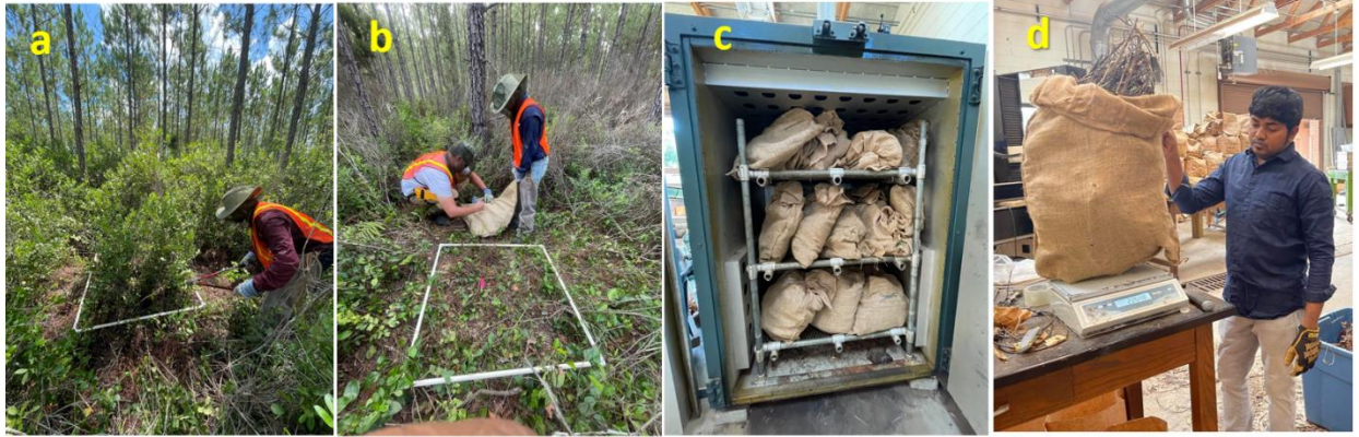
Figure 3.4: The process for collecting understory samples and measuring their dry biomass. First, a 1m 2 PVC frame was used to establish an understory subplot (a). Then, after conducting destructive sampling, the samples were placed in bags and labeled (b). Next, the collected samples were dried in an oven (c) for 48 hours at 105°C before dry biomass weight measurement (d).
