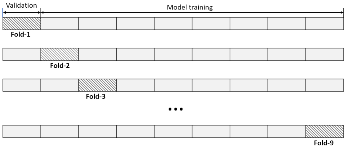
Figure 2.2 The illustration of the 9-fold cross-validation. The dataset is divided into nine random subsets; from there, eight are used for training and one for validation. This process is repeated nine times with different subsets for validation.
