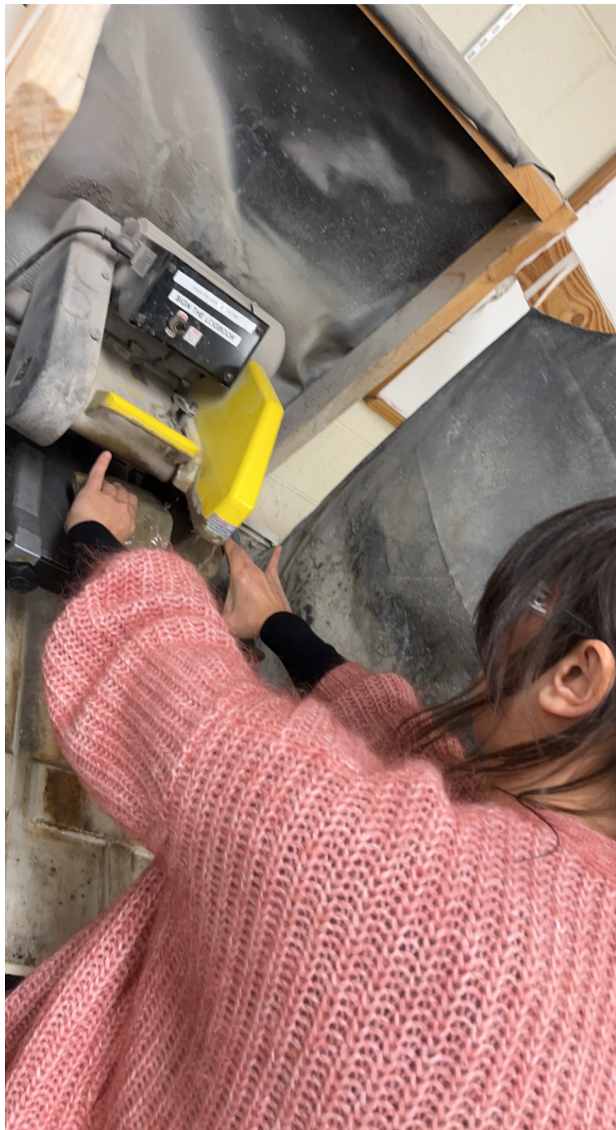
Figure A.1: Cutting rock samples using diamond saw blade.
