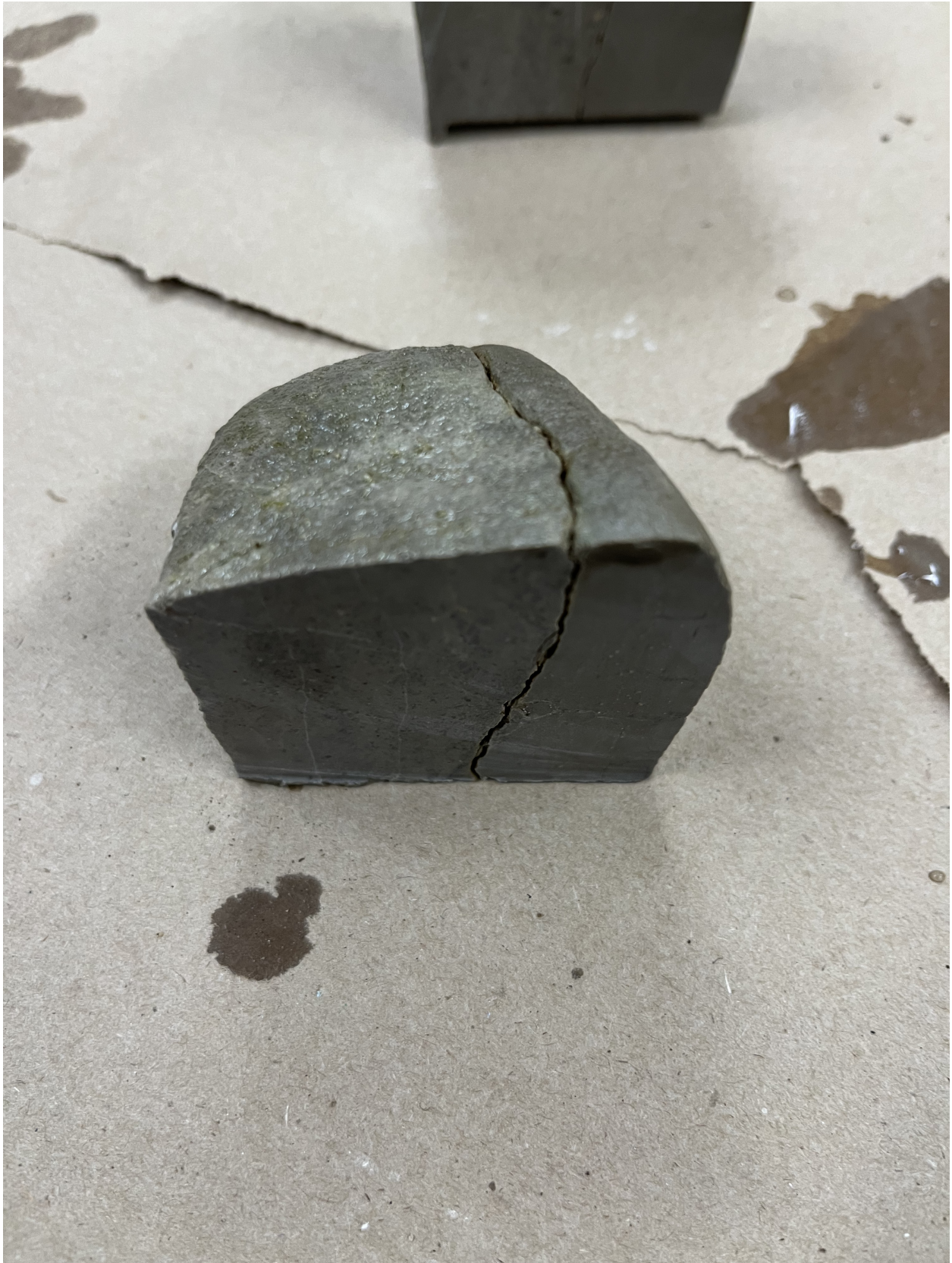
Figure A.5: Fracture exposed from cutting rock.
