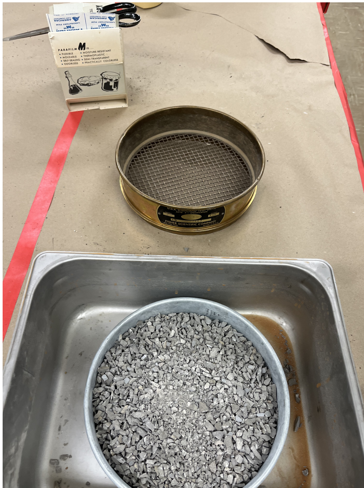
Figure A.4: Crushed rock samples passing through 0.67-cm sieve.
