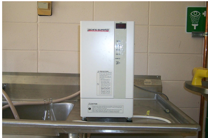
Figure 5. Primacide mixed oxidant generator with the door closed.
