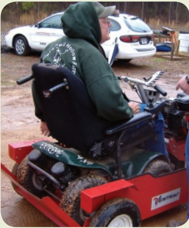
Andy tries out the Ventrac 300. This unique piece of equipment allows users to stay in their own wheel chair by easily rolling into the operating platform. Various attachments are available that enable the farmer to do tasks around the farm.
