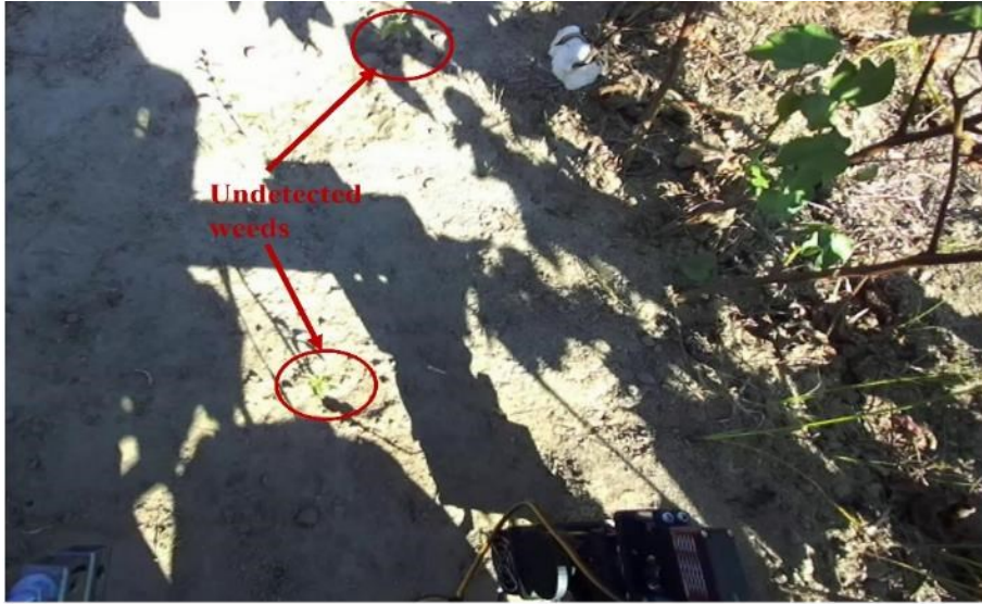
Figure 6.13. Sunlight brightness and shadows hindering weed detection
