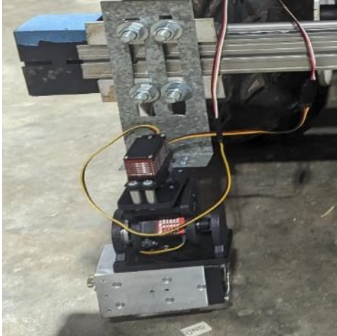
Figure 6.21. Diode laser setup parallel to the ground
