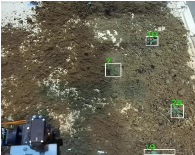
Figure 6.26. Tracking assigning IDs to the weeds
