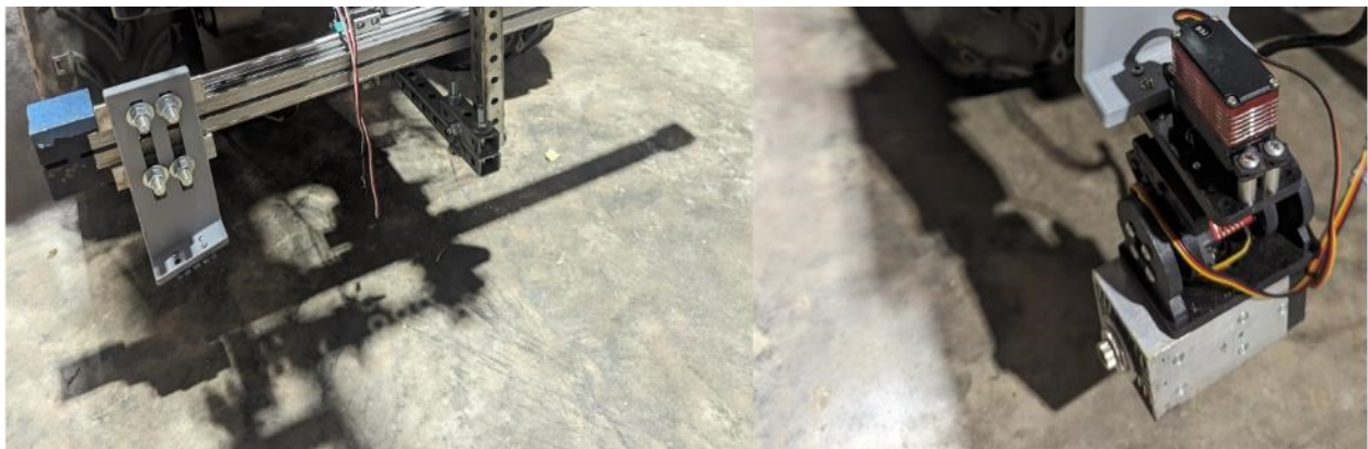
Figure 6.22. The laser module attachment at an angle, and the laser module attached to it
