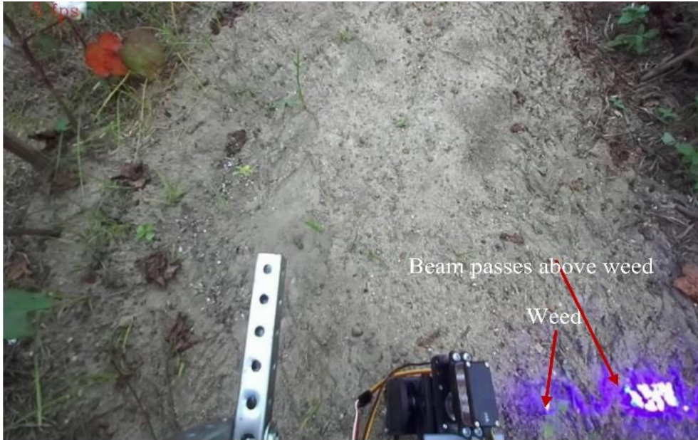
Figure 6.23. Laser beam turned on and slightly misses the weed stem
