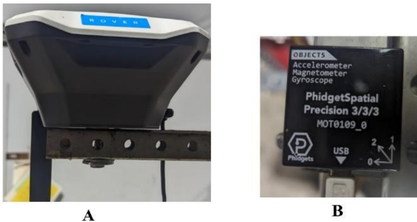
Figure 6.3. GPS receiver (A) and IMU (B) used in the platform
