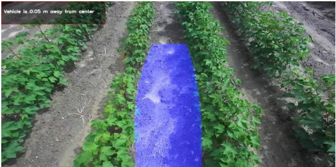
Figure 6.14. Path detected between cotton rows and mapped to the ground plane
