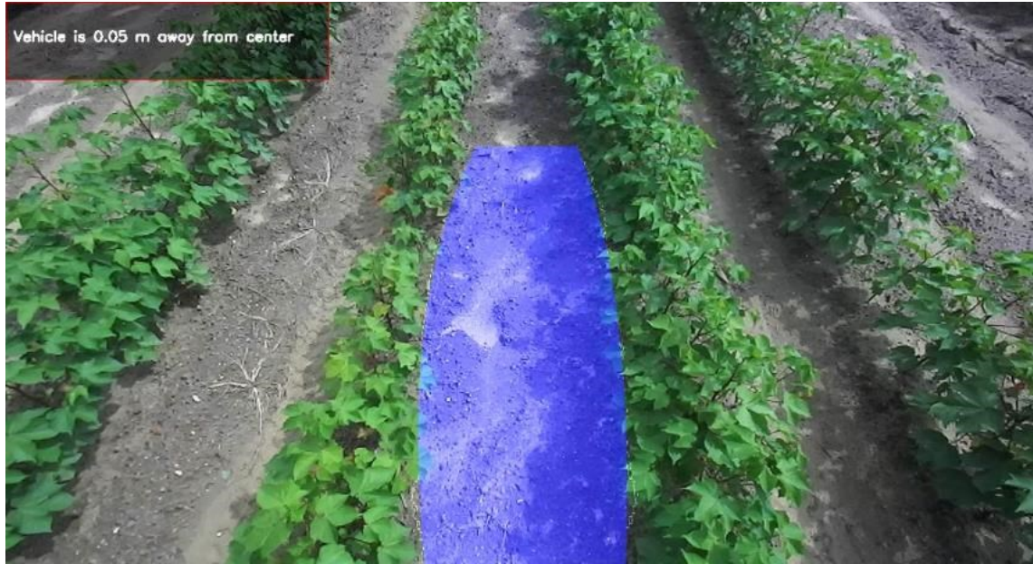
Figure 5.22. Path detected between cotton rows and mapped to ground plane.
