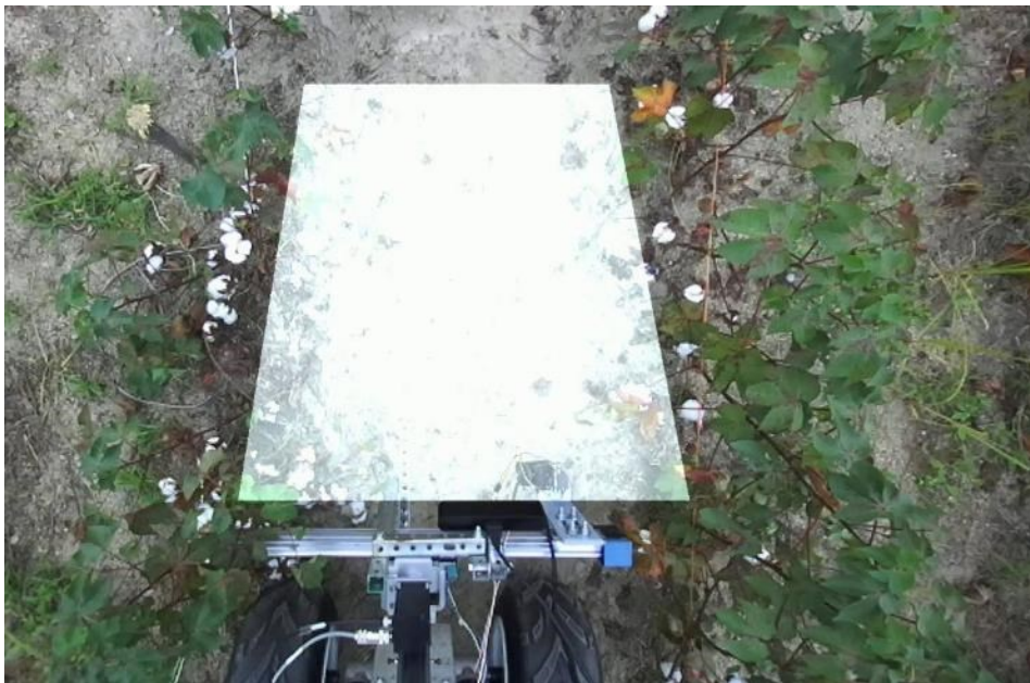
Figure 6.16. Path between cotton rows detected by FCN
