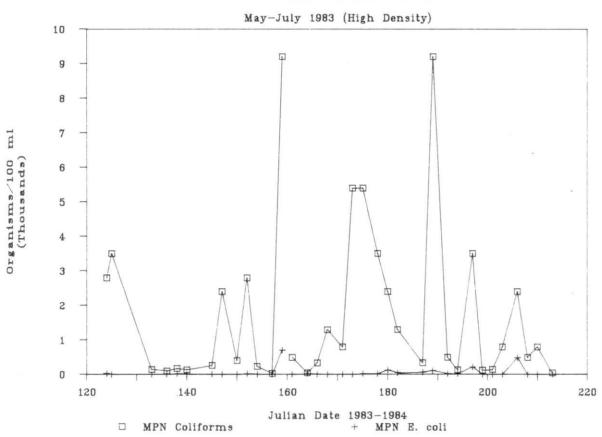
Figure 13. MPN total coliform and MPN  $\underline{E}$ .  $\underline{coli}$  outlet populations for the biological filter stocked at high densities (May-July, 1983)
