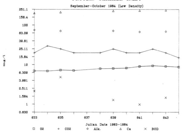
Figure 19. Mean inlet dissolved  $\mathrm{O}_2$ , dissolved  $\mathrm{CO}_2$ , alkalinity, calcium, and BOD levels for the protein skimmer stocked at low densities (September-October, 1984)
