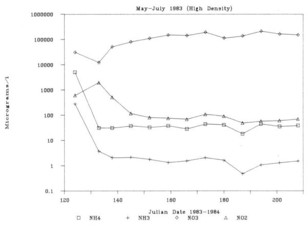
Figure 8. Mean outlet ammonium (NH $_4$ ), ammonia (NH $_3$ ), nitrate (NO $_3$ ), and nitrite (NO $_2$ ) levels for the biological filter stocked at high densities (May-July, 1983)
