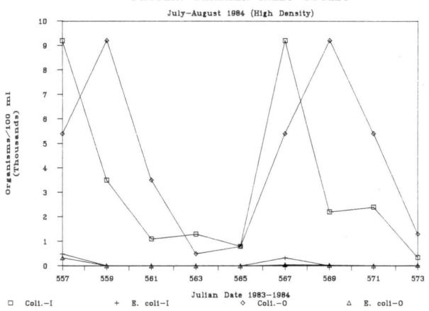
Figure 29. MPN total coliform and MPN <u>E. coli</u> inlet and outlet populations for the protein skimmer stocked at high densities (July-August, 1984)
