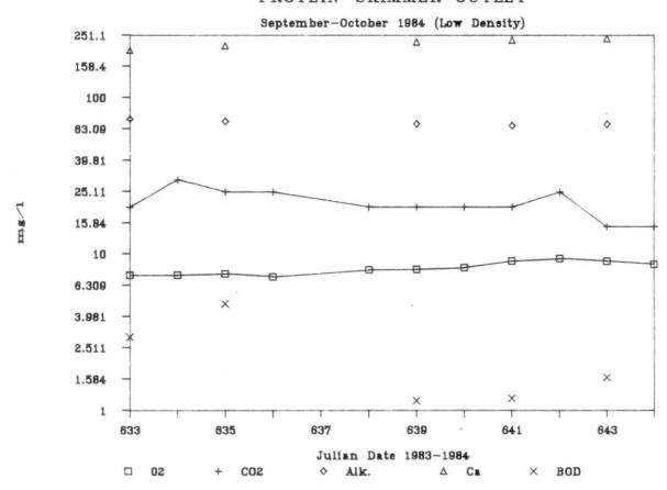
Figure 20. Mean outlet dissolved O<sub>2</sub>, dissolved CO<sub>2</sub>, alkalinity, calcium, and BOD levels for the protein skimmer stocked at low densities (September-October, 1984)
