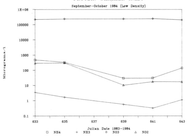
Figure 25. Mean inlet ammonium (NH $_4$ ), ammonia (NH $_3$ ), nitrate (NO $_3$ ), and nitrite (NO $_2$ ) levels for the protein skimmer stocked at low densities (September-October, 1984)
