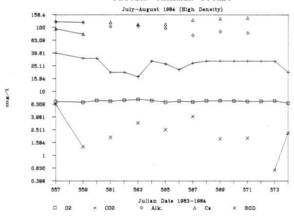
Figure 18. Mean outlet dissolved O<sub>2</sub>, dissolved CO<sub>2</sub>, alkalinity, calcium, and BOD levels for the protein skimmer stocked at high densities (July-August, 1984)
