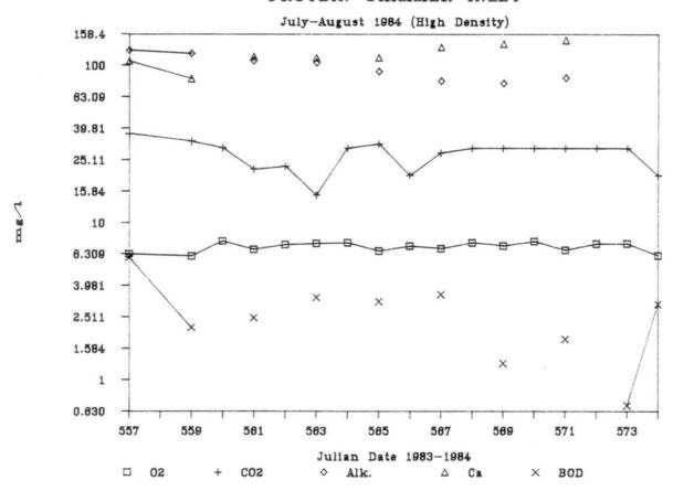
Figure 17. Mean inlet dissolved  $\mathrm{O}_2$ , dissolved  $\mathrm{CO}_2$ , alkalinity, calcium, and BOD levels for the protein skimmer stocked at high densities (July-August, 1984)
