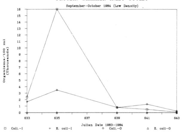
Figure 30. MPN total coliform and MPN <u>E. coli</u> inlet and outlet populations for the protein skimmer stocked at low densities (September-October, 1984)
