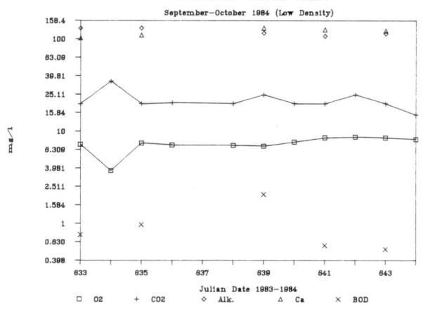
Figure 4. Mean inlet dissolved 02, dissolved C02, alkalinity, calcium, and BOD levels for the biological filter stocked at low densities (September-October, 1984)
