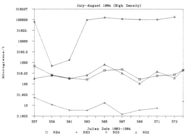
Figure 24. Mean outlet ammonium (NH $_4$ ), ammonia (NH $_3$ ), nitrate (NO $_3$ ), and nitrite (NO $_2$ ) levels for the protein skimmer stocked at high densities (July-August, 1984)
