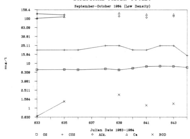
Figure 5. Mean outlet dissolved  $0_2$ , dissolved  $0_2$ , alkalinity, calcium, and BOD levels for the biological filter stocked at low densities (September-October, 1984)
