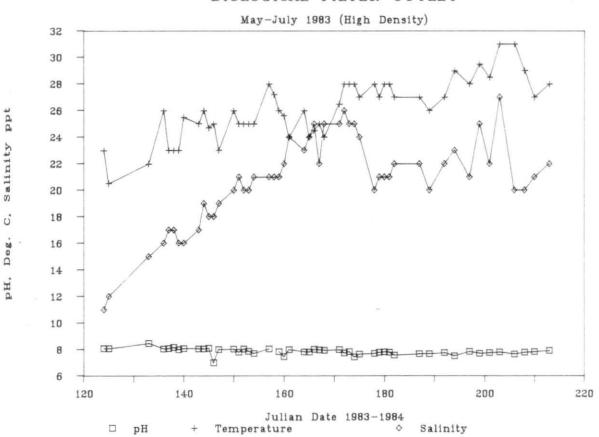
Figure 1. Outlet pH, temperature (°C), and salinity (ppt) levels for the biological filter stocked at high densities (May-July, 1983)
