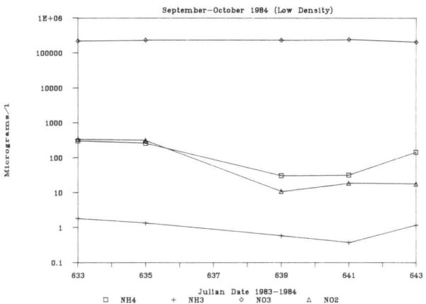
Figure 26. Mean outlet ammonium (NH $_4$ ), ammonia (NH $_3$ ), nitrate (NO $_3$ ), and nitrite (NO $_2$ ) levels for the protein skimmer stocked at low densities (September-October, 1984)
