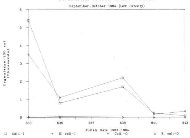
Figure 14. MPN total coliform and MPN <u>E. coli</u> inlet and outlet populations for the biological filter stocked at low densities (September-October, 1984)
