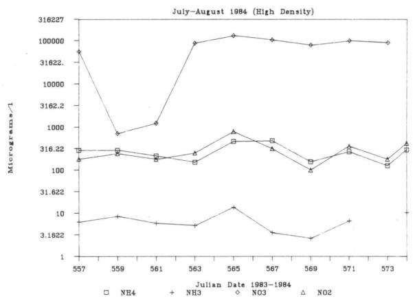
Figure 23. Mean inlet ammonium ( $\mathrm{NH_4}$ ), ammonia ( $\mathrm{NH_3}$ ), nitrate ( $\mathrm{NO_3}$ ), and nitrite ( $\mathrm{NO_2}$ ) levels for the protein skimmer stocked at high densities ( $\mathrm{July-August}$ , 1984)
