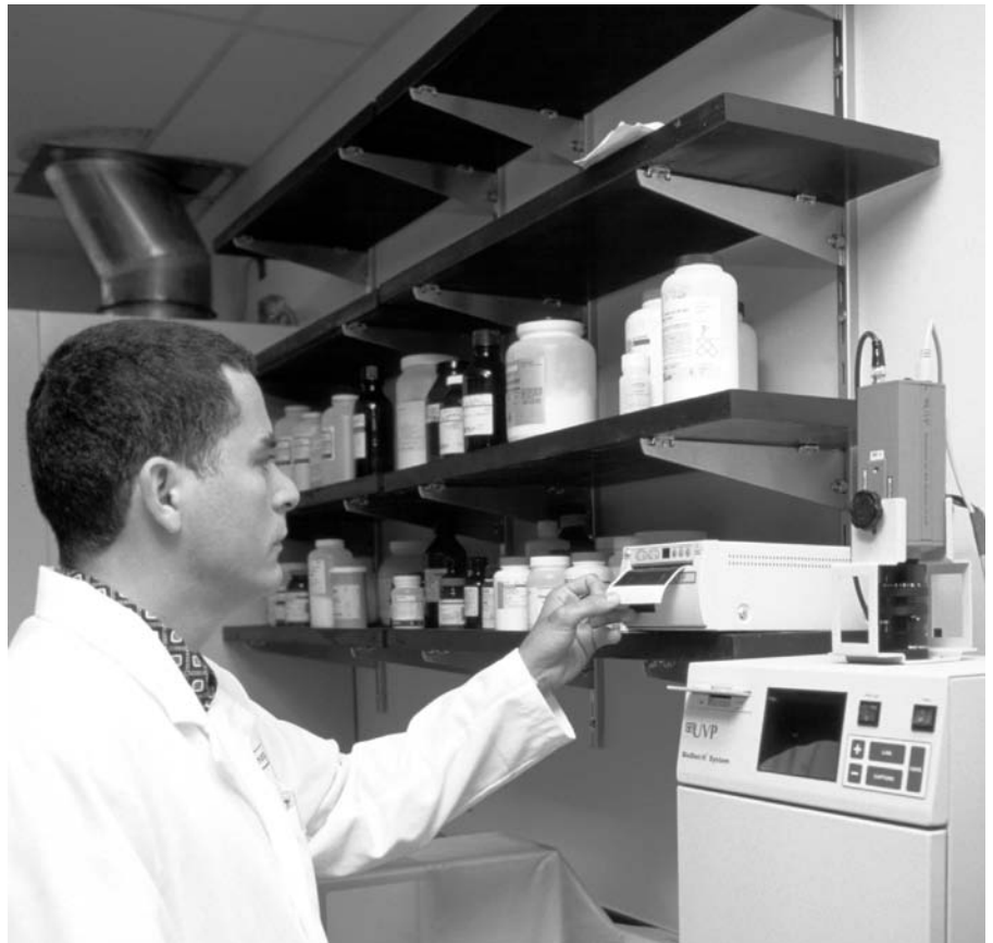
Dr. Carlos Estevez uses the UVP Biodoc-IT System for rapid and accurate analysis of DNA migration patterns in an agarose gel following electrophoresis.
