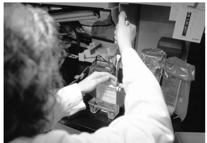
A graduate student in Dr. Maricarmen García's laboratory loads an electrophoretic gel apparatus during an experiment to characterize the genome of avian viruses.
