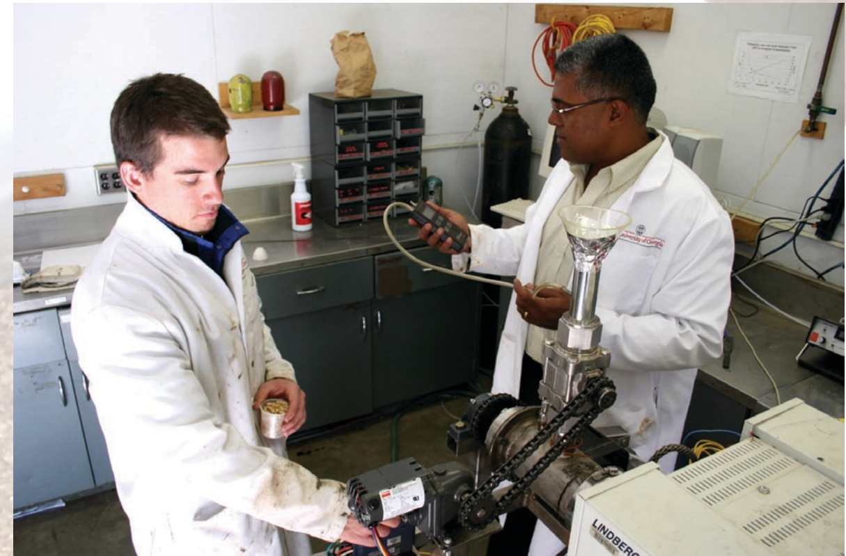
Brian Bibens and K.C. Das check the process of the continuous pyrolysis machine. They will use pyrolysis to turn coarse particles of chicken litter into char and bio-oil.
